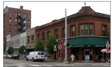
Arrange windows in patterns that will reinforce the rhythm and alignment of windows on adjacent historic structures and in the surrounding historic district.
