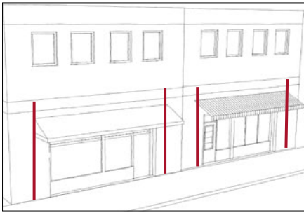
When using canopies on new construction in historic commercial settings, special emphasis should be placed on sizing and positioning canopies to reflect the traditional storefront rhythm seen on adjacent historic structures and in the surrounding historic district.
