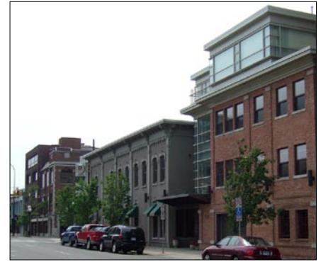
Although creative and contemporary designs are encouraged, the apparent solid-to-void ratios seen on the primary facades of adjacent historic structures should be maintained.
