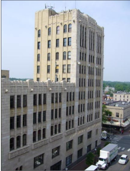
Taller historic structures in downtown Ann Arbor respect the surrounding streetwall pattern. Taller portions are seen to be compatible with smaller buildings in the area because first floors are articulated to express this traditional scale.
