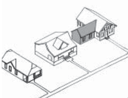
Side addition – NOT Recommended
