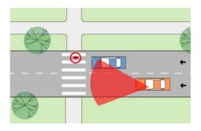
2. The driver closest to the pedestrian lane stops, yielding the right-of-way to the pedestrian. The car is stopped immediately adjacent to the crosswalk, therefore blocking the sightlines between the pedestrian and the driver of the other car.
