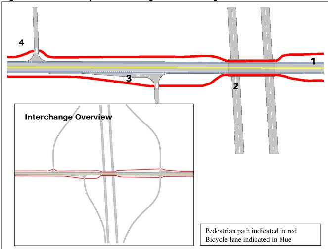
Fig. 2.4K. Urban Overpass Interchange Retro-fit Design Guidelines
