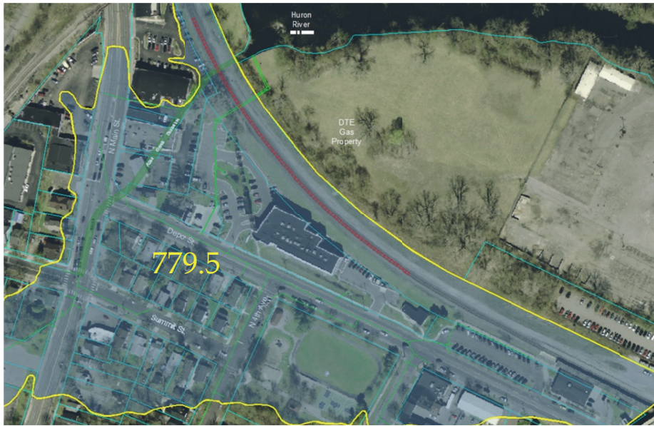
Figure 11 Existing Floodplain (Official FEMA Floodplain Elevation)
