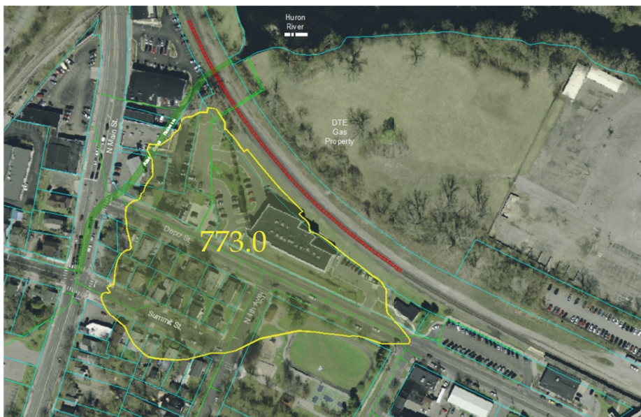
Figure 12 Floodplain After Proposed Improvements
