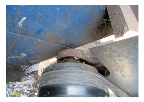
Photos A & B show the condition of the bearings. We recommend that both head shaft bearings are replaced as soon as possible.
