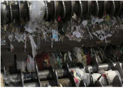
Photos A & B show the worn condition of the rotors. We recommend replacing these rotors to increase the separation performance of this screen. We also recommend removing the wrappings from the rotors on a regular basis to insure maximum separation performance and to prevent material jams.
