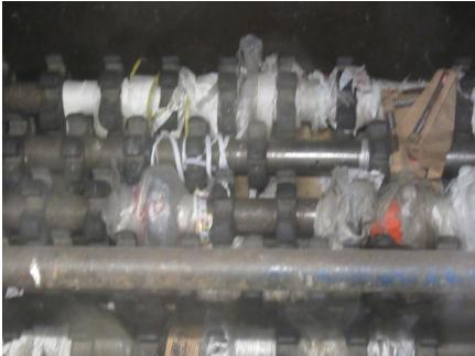
Photos A & B show the worn and missing finger discs. These discs are crucial to maximizing the material separation for this screen. We recommend replacing all of the finger discs on this screen. Also, the photos show the excessive amount of wrappings on the rotors. We recommend removing the wrappings on a regular basis to help maximize material separation.
