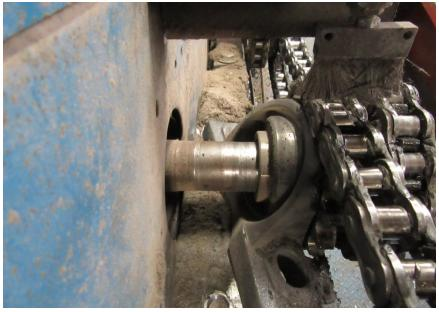
Photos A & B show damage to the bearings. These damaged bearings are a result of the misaligned rotors. Out of time rotors can cause material jams, damaging the bearings as shown. We recommend that the rotors are properly clocked on a regular basis to prevent this problem.
