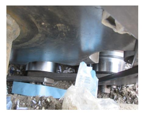
Photos A & B show the lack of tensioning on the belt. We recommend tensioning the belting on a regular basis to prevent premature wear of the belting and sprockets.
