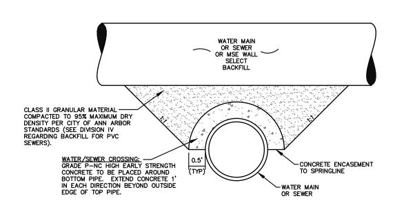
APPLIES TO: WATER AND/OR SEWER CROSSINGS WITH LESS THAN 1.5' OF VERTICAL CLEARANCE
