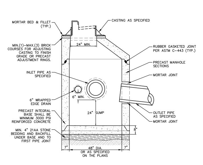
1. FRONT EDGE OF INLET CASTING SHALL BE FLUSH WITH FRONT EDGE OF GUTTER (EDGE-OF-METAL)
