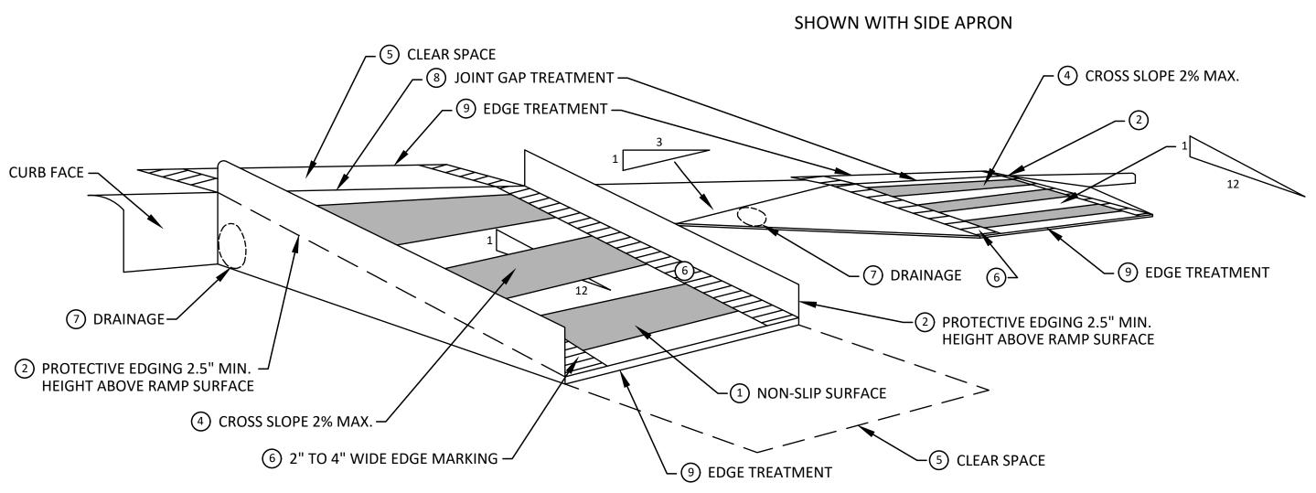
TEMPORARY CURB RAMP PERPENDICULAR TO CURB
