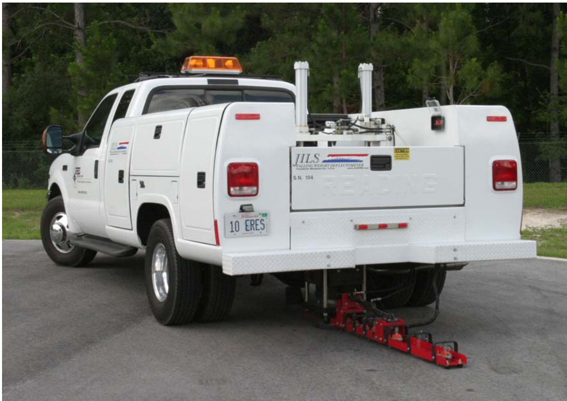
Figure 1. The JILS truck-mounted FWD configured with nine deflection sensors.
