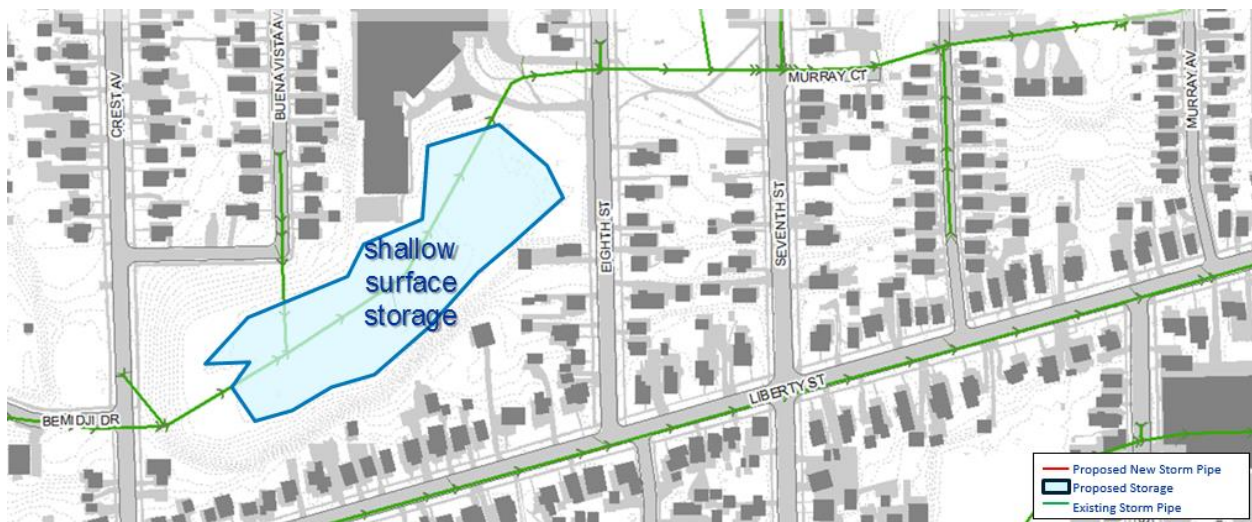
Figure 4-27 – Conceptual Layout for Surface Storage Alternative for Mulholland Ave
