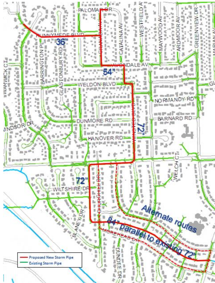
Figure 4-17 – Conceptual Layout for Conveyance Alternative for Churchill Downs
