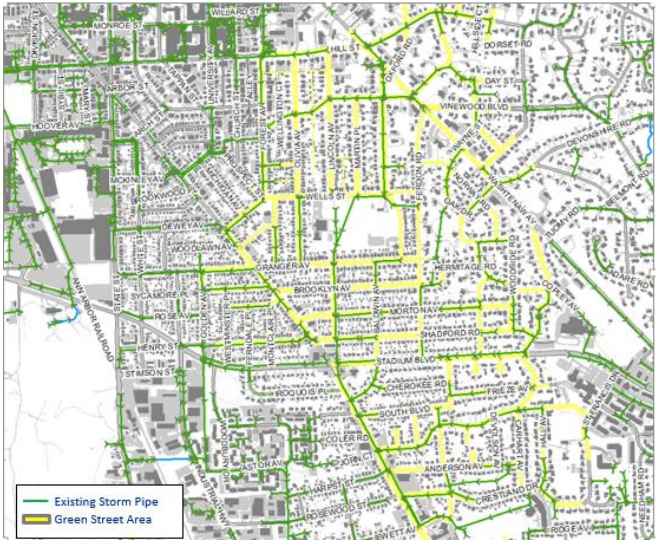
Figure 4-51 – Conceptual Layout for Green Streets Alternative for S. Industrial Area
