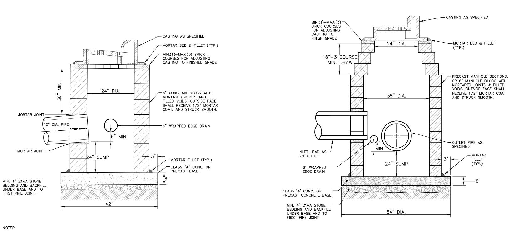
1. MAY BE USED WITH ONLY SINGLE OUTLET PIPE, AND NO INLET PIPE
