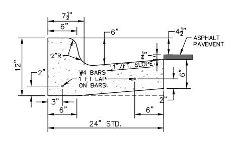
CURB AND GUTTER, CONC, DET F4, SPECIAL NO SCALE
