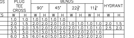
FOR FITTING SIZES LARGER THAN 16", THRUST BLOCK DIMENSIONS SHALL BE AS SPECIFIED BY ENGINEER.
