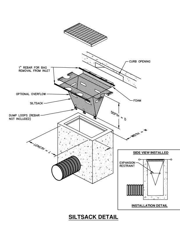
NOTE: THE SILTSACK WILL BE MANUFACTURED FROM A WOVEN POLYPROPYLENE
