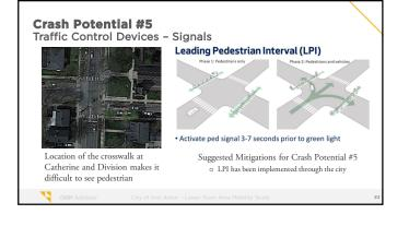
In the specific case of Catherine at Division, the irregular shape of the intersection could result in turning traffic not being fully aware of pedestrians crossing 'on the green' as they should.
