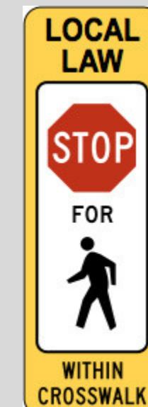
In-Lane Signs (R1-6a)
