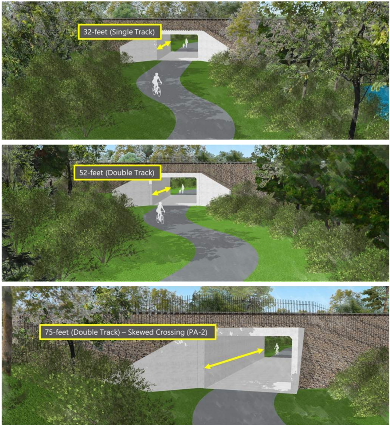
Exhibit 1-19: Comparison of Single vs. Double Track Underpass Length
