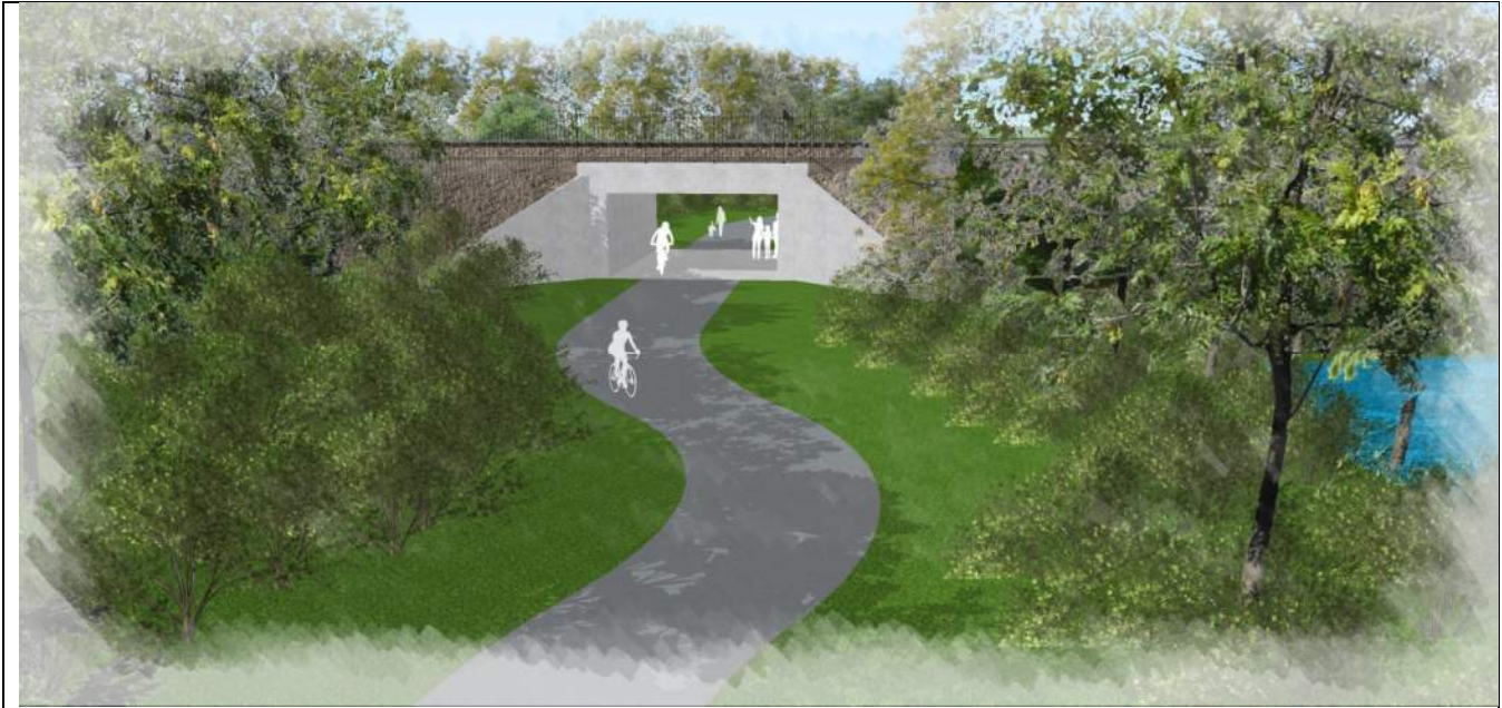
Exhibit 1-13: Rail Bridge (ST-2) Showing a Single-Span Concept Looking South (20-foot span shown)
