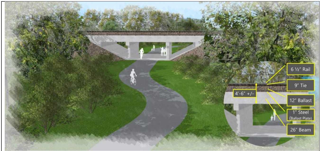
Exhibit 1-15: Rail Bridge (ST-2) Showing a 3-Span Concept Looking South (20-foot wide main span shown)
