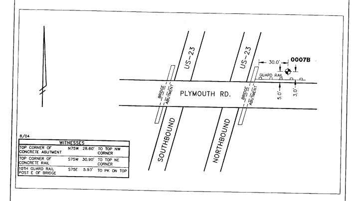
STATION 0007B IS LOCATED ON THE NORTH SIDE OF PLYMOUTH ROAD, EAST OF THE US-23 BRIDGE, SAID STATION BEING IN THE SOUTHEAST 1/4 OF SECTION 14, ANN ARBOR TOWNSHIP, MICHIGAN. THE STATION IS LOCATED 30' EAST OF THE EAST EDGE OF THE EAST EDGE ABUTMENT AND 3' NORTH OF THE GUARDRAIL ALONG THE NORTH SIDE OF PLYMOUTH ROAD. SAID STATION IS A PRIMARY CONTROL STATION AND IS DESCRIBED AS THE 1993 EDITION OF THE CITY OF ANN ARBOR IN 1993 AND IS PAIRED WITH STATION 0007A.
