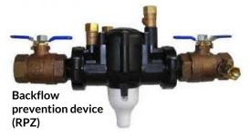
Water powered backup pumps are installed with a backflow prevention device, also known as a reduced pressure zone (RPZ) valve, to prevent sump pump water from entering the municipal water supply.
