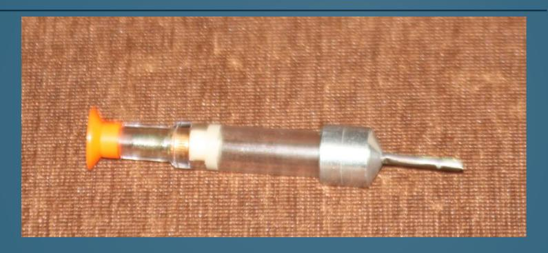
For opportunistic remote delivery, a customdesigned dart was created to inject the liquid primer/time-release pellets and then eject from the targeted animal's body
