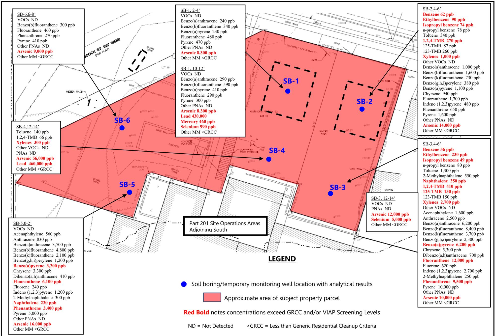
**Figure 2: Soil Boring Locations with Soil Analytical Results**
