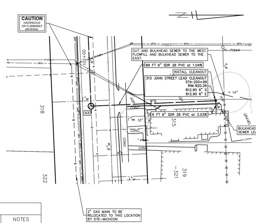
2" GAS MAIN TO BE RELOCATED TO THIS LOCATION BY DTE-MICHCON
