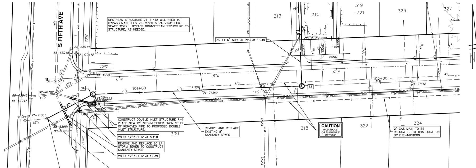
UPSTREAM STRUCTURE 71-71412 WILL NEED TO BYPASS MANHOLES 71-71380 & 71-71411 FOR SEWER WORK. BYPASS DOWNSTREAM STRUCTURE TO STRUCTURE, AS NEEDED.
