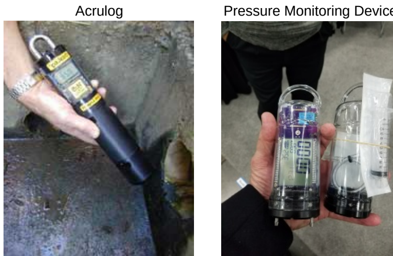
Figure 2-1. Acrulog and Pressurization Testing Gear
