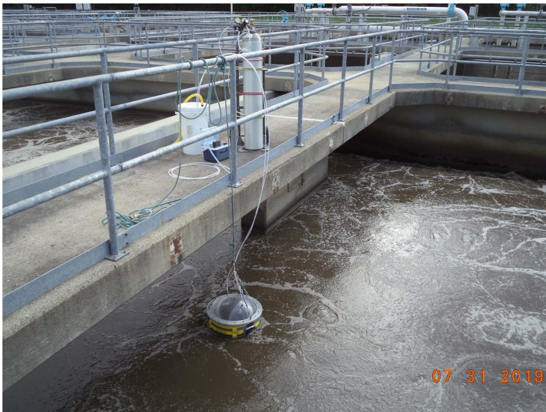
FIGURE 1: SUMMER SAMPLING USING AN EPA FLUX CHAMBER
