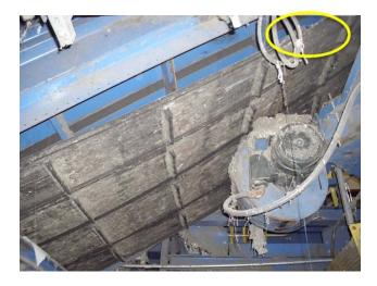
Belt is torn and needs to be replaced. Tensioning is lacking.
