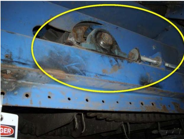
Pulleys, bearings and guarding is damaged. Replacement of all components required.
