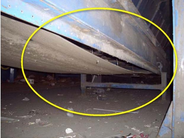
Tensioning is lacking, return rollers omitted. Replacement of rollers required.
