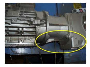
Gearmotor is leaking. Replacement required.
