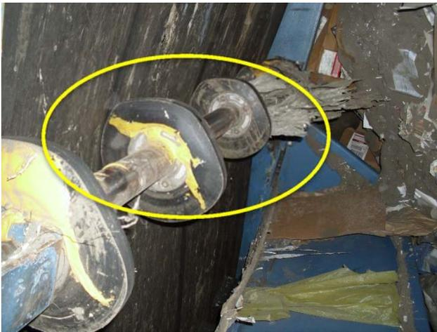
Return rollers are worn and needs to be replaced.
