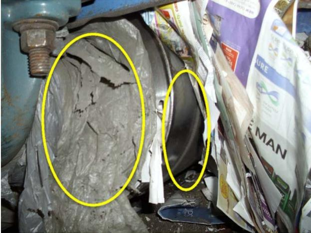
Shaft is wrapped, belt tracking needs to be corrected.
