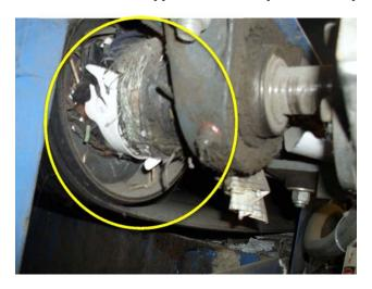
Pulley shafts are wrapped, bearings are worn, replacement of all required.
