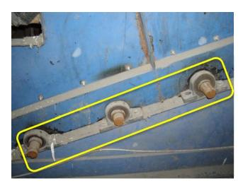
Shafts should be better aligned to normalize disk spacing.
