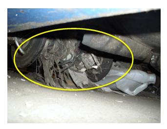
Return rollers need to be replaced. Some return rollers are missing/omitted.
