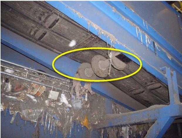
Return rollers are worn and need to be replaced.
