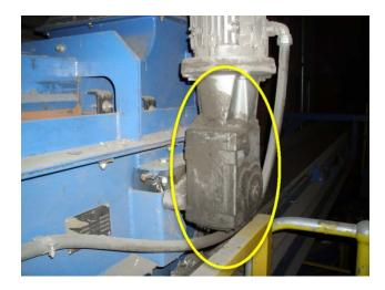
$Gearmotor\ is\ leaking, replacement\ required.$
