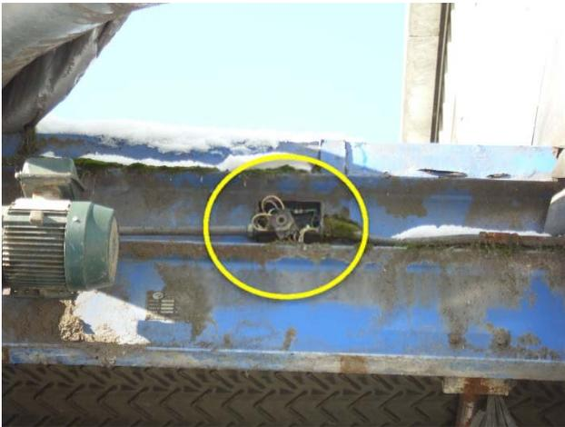
Disconnect switch is missing.
