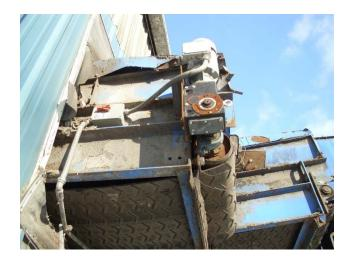
Wire wrapped around pulley and shaft.
