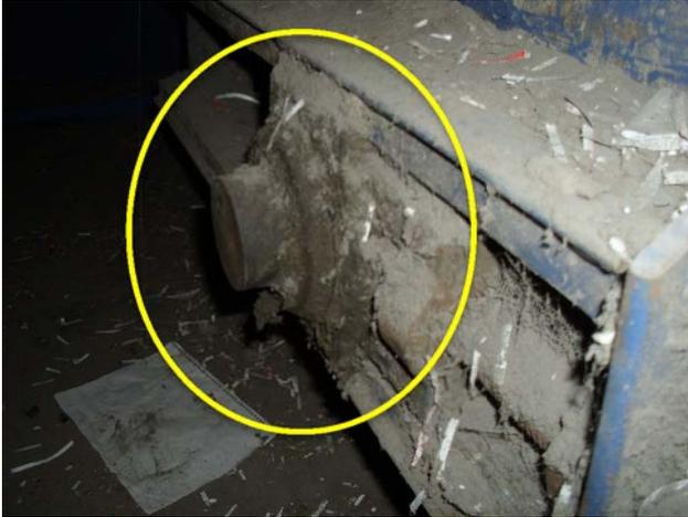
Both head and tail pulley and bearings are severely worn, replacement required.
