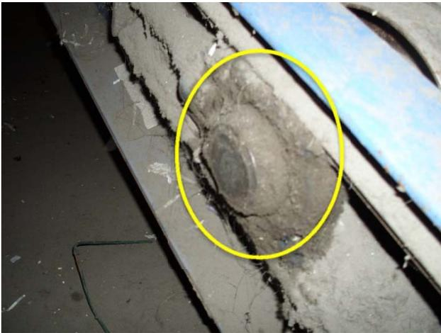
Bearings are worn/broken, replacement required.
