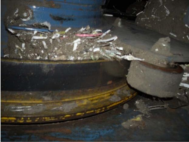
Guards are omitted/missing, motor is leaking, replacement required.
