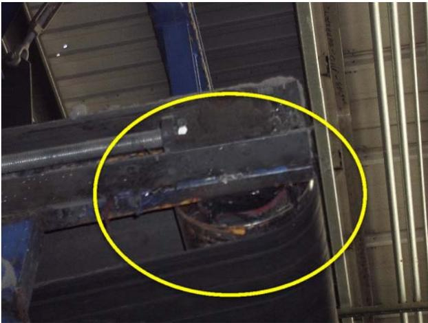
Picture shows severely worn pulleys and bearings.
