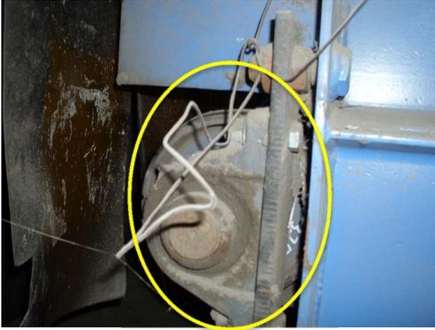
Bearing is worn, tracking of belt veers to the right, replacement required.
