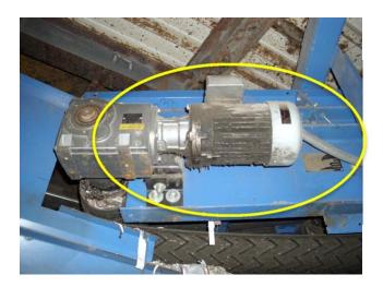
Gearmotor is leaking, replacement required.
