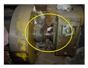
Bearings and gearmotor need to be replaced.
