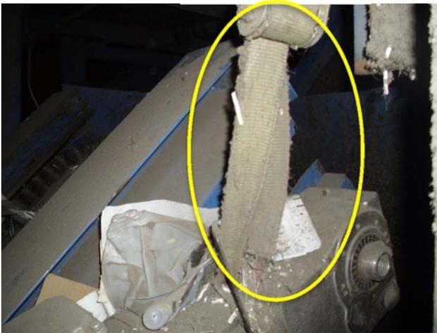
Gearmotor is leaking. Torque arm needs to be replaced as motor is held up by a tie down.
