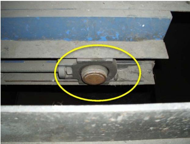
Bearings are worn, replacement required.
