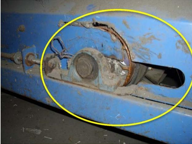
Pulley is worn, bearing is worn, guarding is damaged, replacement of all required.
