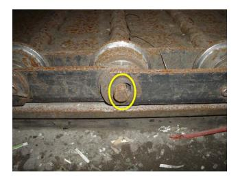
D hole bars are worn out, no cotter pin installed.
