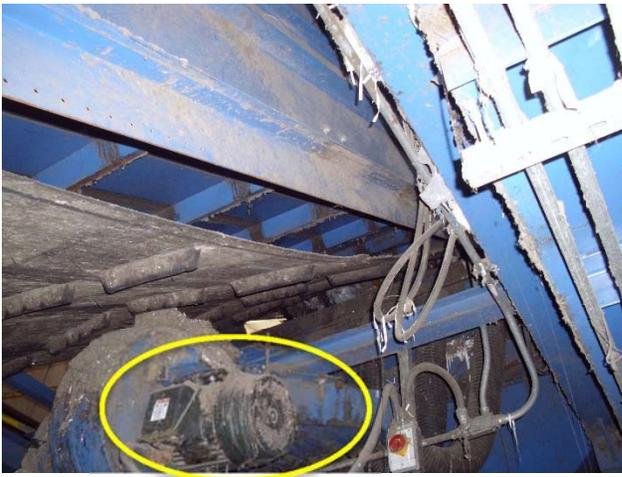
Gearmotor is leaking and needs to be replaced.
