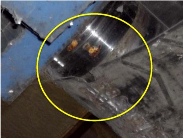
Pulley needs to be replaced. Belt is not tracked properly. Lacing is damaged and caused belt to tear.
