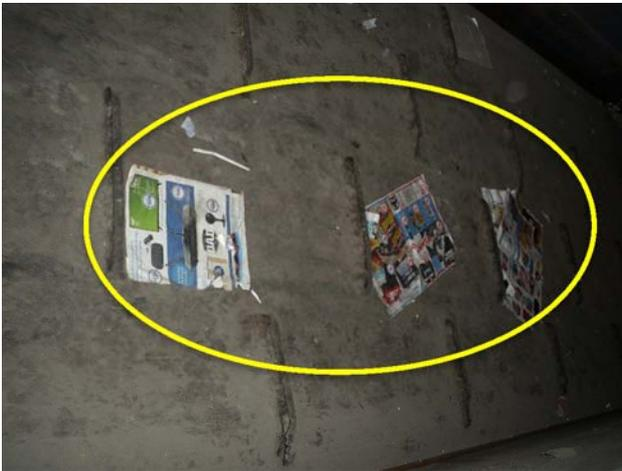
Belt is worn, cleats are barely visible, replacement required.
