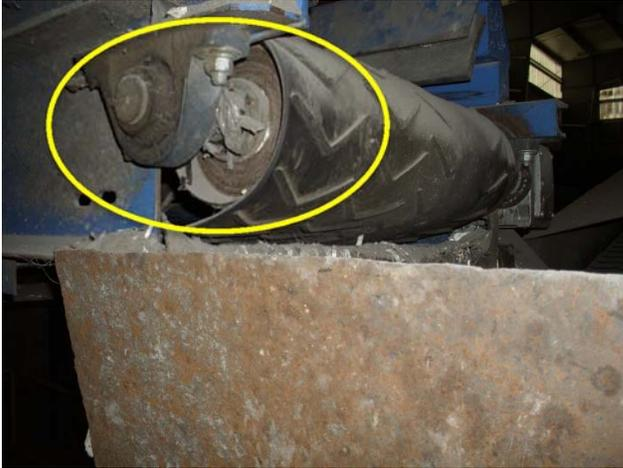
Pulleys and bearings are damaged, replacement required.
