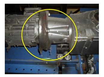
Gearmotor is leaking, replacement required.
