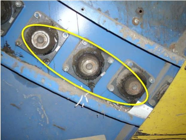
Bearings are worn and need to be replaced.
