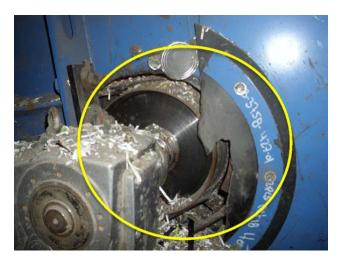
Lagging on pulley is worn, replacement required.
