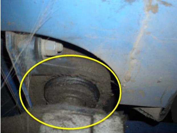
Bearings are worn, replacement required.
