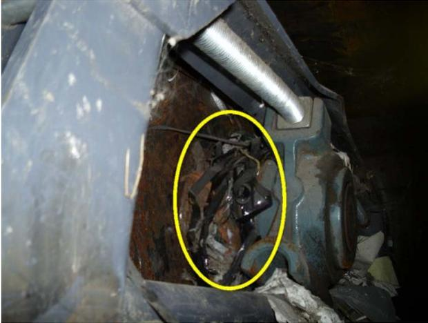
Picture shows wrapped shafts. Take up frame is bent.
