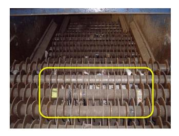
Shafts need wrapping removed and cleaned.
