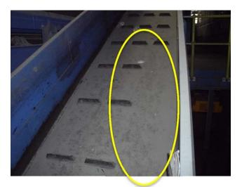
Belt is worn and need to be replaced. Missing cleats.
