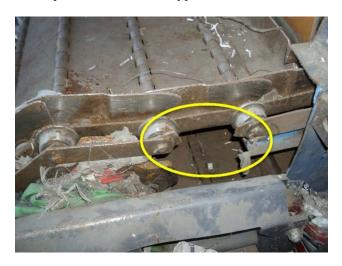
D hole bars are missing/broken.
