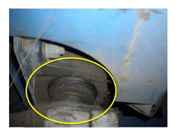
Bearings are worn, replacement required.
