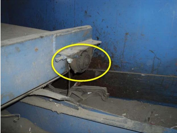
Bearing is worn, replacement required.
