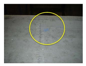
Belt is torn, lacing torn, replacement required.
