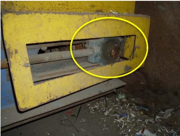
Bearings are worn/blown, replacement required.
