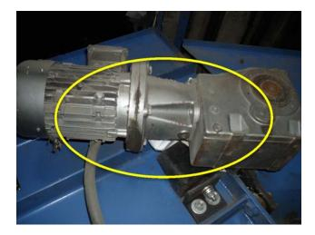
Gearmotor is leaking, replacement required.
