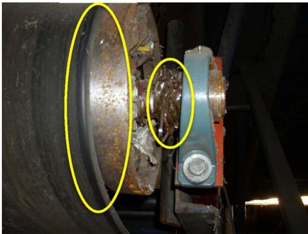
Above picture shows the condition of the belt tracking. It also indicates the condition of the pulley and the shaft being wrapped.
