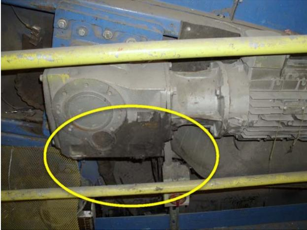
Gearboxes on all decks are leaking and needs to be replaced.
