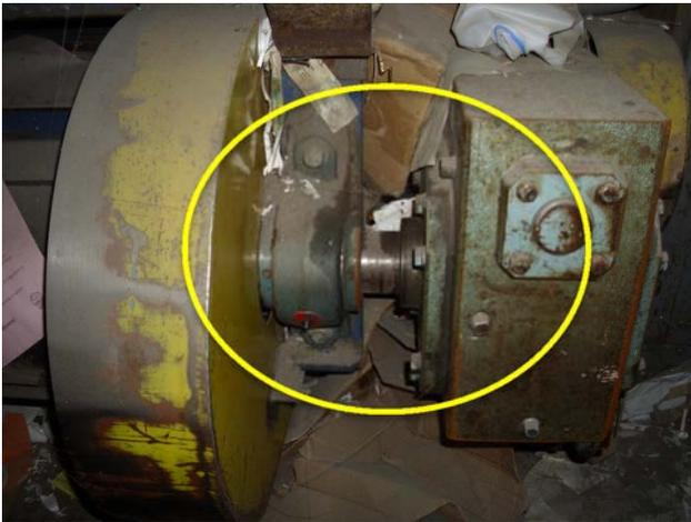
Bearings and gearmotor need to be replaced.
