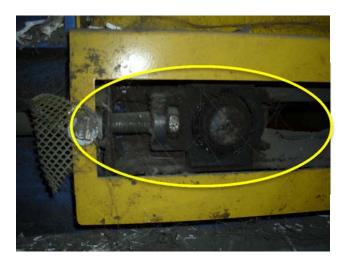
Bearing is worn, guarding is omitted, replacement required.
