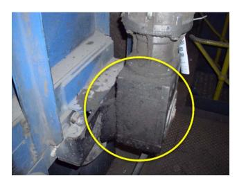
$Gearmotor\ is\ leaking, replacement\ required.$
