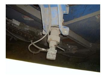
Hydraulic Lines needs to be replaced and/or fixed.
