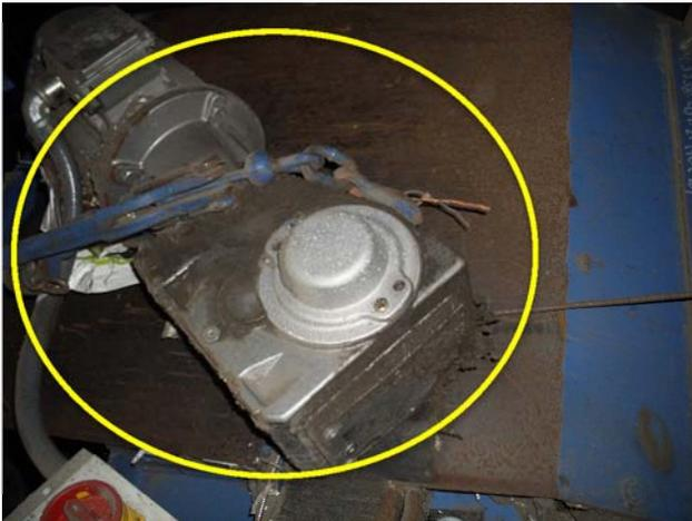
Gearmotor is not secured safely and is leaking, replacement required.
