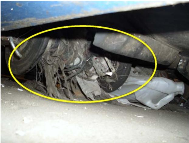
Return rollers need to be replaced. Some return rollers are missing/omitted.
