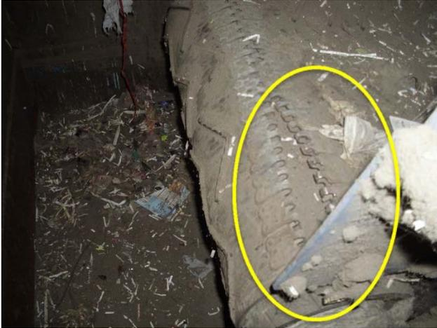
Belt is torn, lacing is ripped, replacement required.
