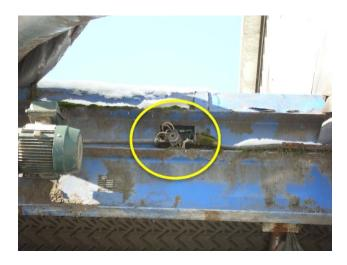
Disconnect switch is missing.
