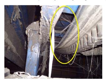
Belt tensioning is off, return rollers required to enhance optimal use.
