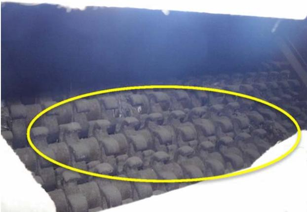
All discs are worn and need to be replaced.
