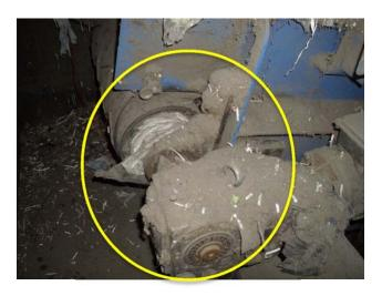
Severely wrapped head shaft, belt tracking is off, gearmotor is leaking. Replace all components.
