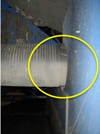
Belt tracking is pulling to the left, belt is worn and needs to be replaced.
