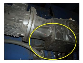
Gearmotor is leaking, replacement required.
