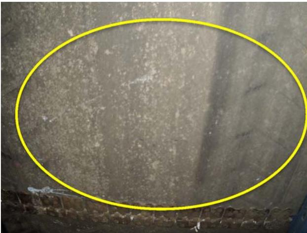
Belt is severely worn, replacement required.
