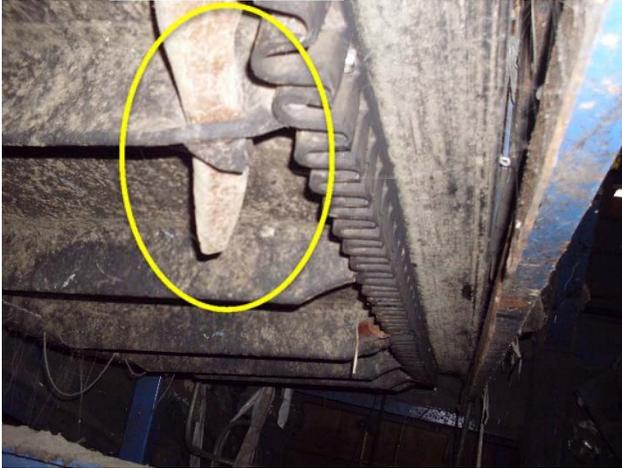
Belt is worn and objects are protruding through cleats, replacement required.
