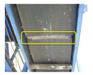
Lacing is damaged. Belt is torn.
