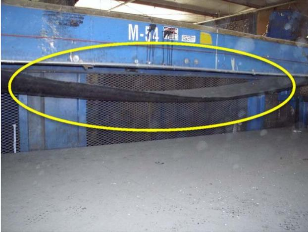
Tensioning is off, belt is not supported by any rollers.
