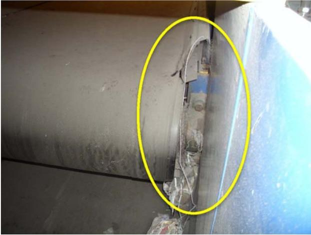
Belt is torn, debris is piled up under belt which is causing the tracking to be off and more strain on the belt.
