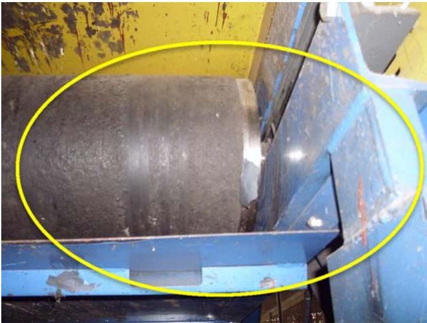
Belt is worn, replacement required. Tracking is off. Pulleys are worn. Bearings are worn.
