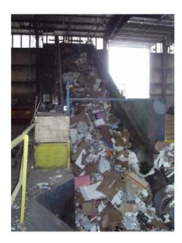
Amount of debris pile up has made it impossible for technician to properly inspect all aspects of the conveyor. It is said that the rails/tracks are worn, head shaft is bent and belt is in bad condition.
