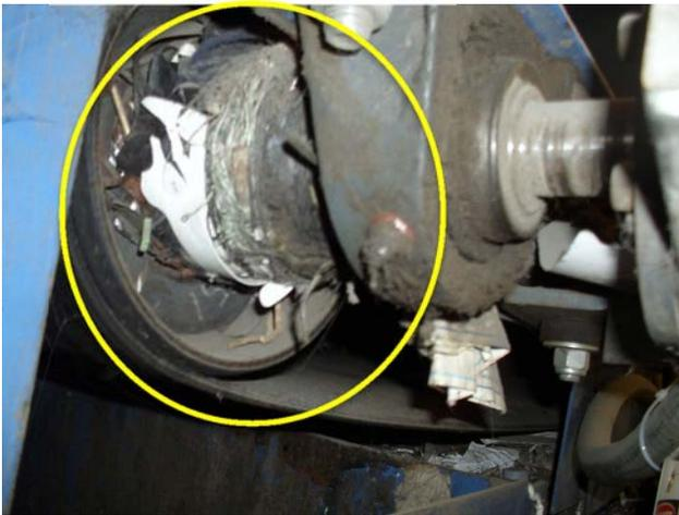
Pulley shafts are wrapped, bearings are worn, replacement of all required.
