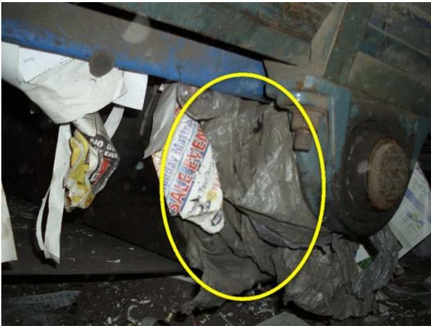
Shafts are wrapped and needs to be cleaned.
