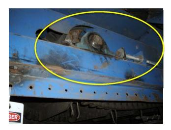
Pulleys, bearings and guarding is damaged. Replacement of all components required.
