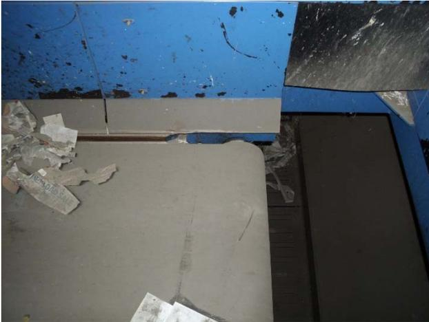
Belt is worn, tracking is off, replacement required.
