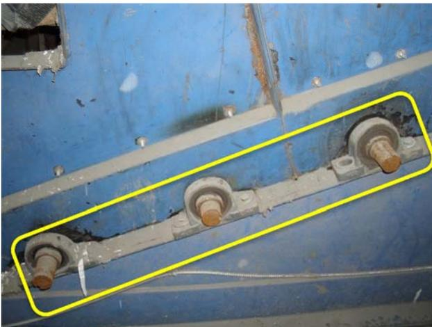
Shafts should be better aligned to normalize disk spacing.
