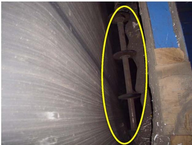
Return Rollers show signs of wear and should be replaced. Head and Tail Pulley needs to be replaced. Overall condition of conveyor is fair, cleaning required for optimal work.
