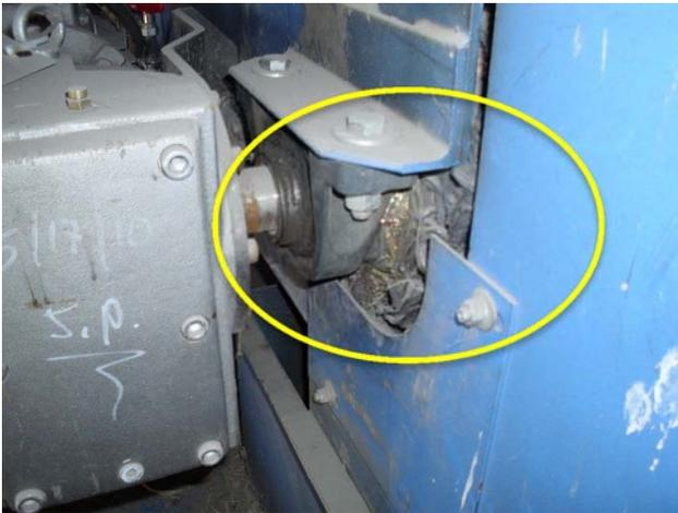
Picture above shows wrapped shaft, cleaning required. Material is building up under belt, causing more damage.
