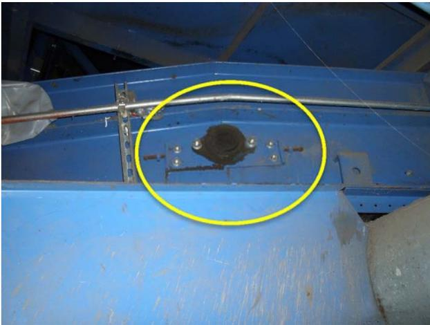
Bearings are worn/blown, replacement required.
