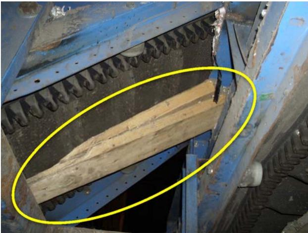
Return rollers are omitted, wood used instead. Immediate replacement required.
