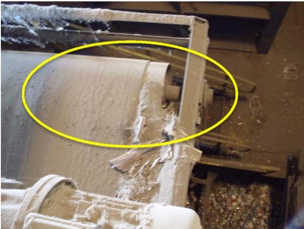
Belt is tracking to the left and is worn, replacement required.
