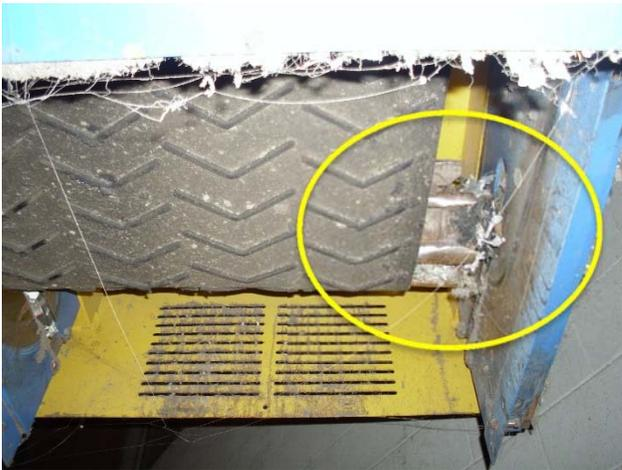
Belt tracking is pulling to the left, pulleys are both damaged beyond repair, replacement of belt, pulleys and bearings recommended.
