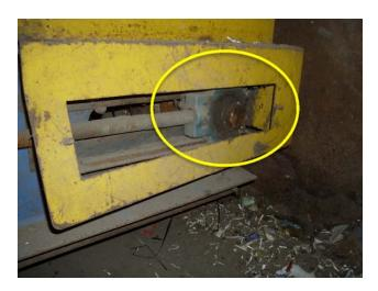
Bearings are worn/blown, replacement required.
