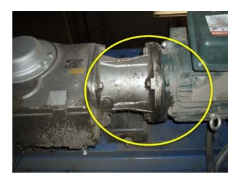
Gearmotor is leaking, replacement required.
