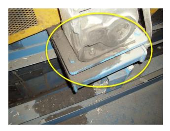
Gearmotor is leaking, replacement required.
