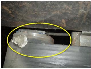
All components on this conveyor need replacement. Both pulleys, bearings, belt, gearmotor, return rollers. Replacement of conveyor recommended.
