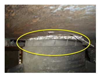
Picture shows belt tracking being off.
