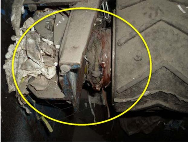
Pulleys are wrapped, replacement required.
