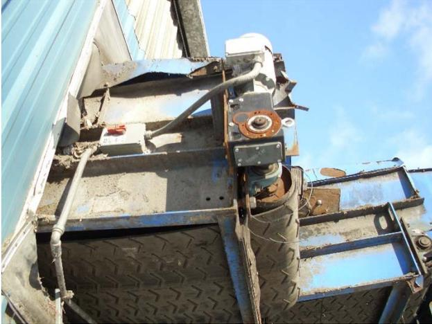
Wire wrapped around pulley and shaft.
