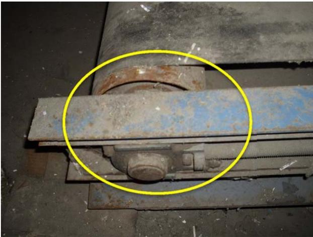
Above picture indicates a severely worn belt, pulley and bearing. Replace all components.
