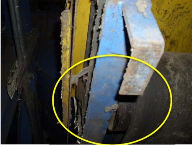
Picture indicates a pulley worn, replacement required. Bearing is worn as well, replacement required.
