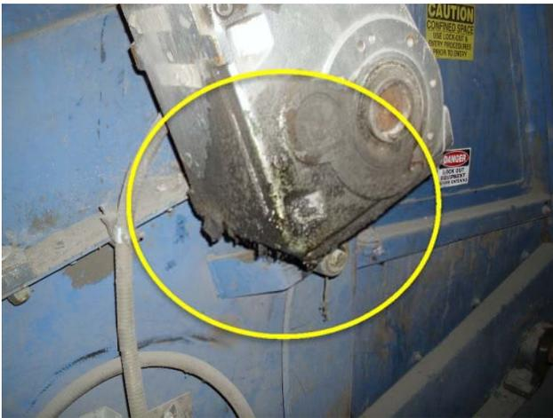
Gearbox is leaking, seal needs to be replaced.
