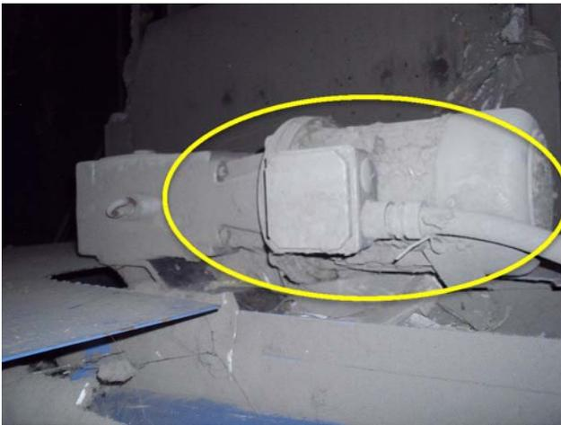
Motor is filled dust and surrounded by debris, replacement required.
