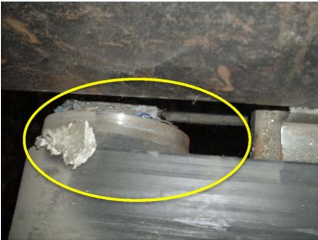
All components on this conveyor need replacement. Both pulleys, bearings, belt, gearmotor, return rollers. Replacement of conveyor recommended.
