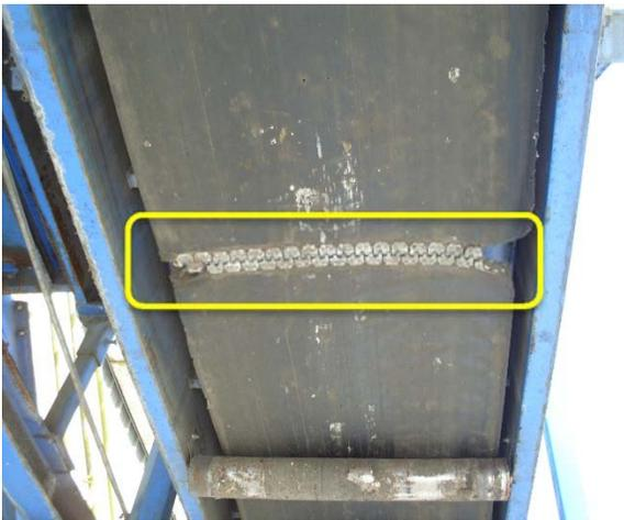
Lacing is damaged. Belt is torn.
