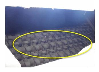
All discs are worn and need to be replaced.
