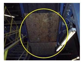
Plywood installed as belly pans, removal required.
