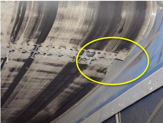
Belt and lacing are torn and needs to be replaced.
