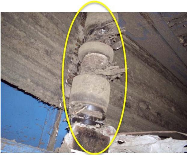
Return rollers are worn and need to be replaced. Picture also indicates a torn and severely worn belt, replacement required.
