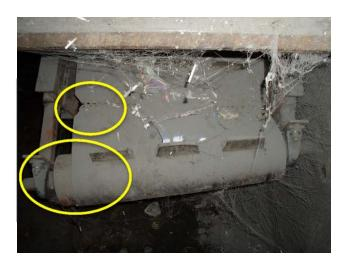
Picture shows belt tracking to the right, lacing and belt torn. Pulleys and bearings need to be replaced.
