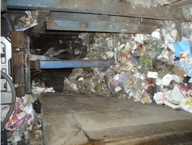
The trash pile up on this conveyor has made it impossible for the technician to do a proper inspection of all components. From the pictures it can be said that this conveyor is in a very worn state and cannot function properly without correction of most components.
