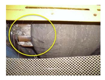
Pulleys are damaged, replacement of pulleys and bearings recommended. Belt tracking is to the right.
