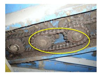
Chains are stretched/worn, full replacement needed. Sprockets are worn, replacement needed.
