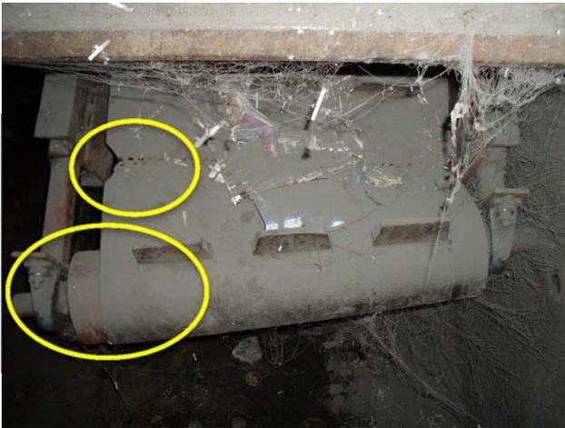
Picture shows belt tracking to the right, lacing and belt torn. Pulleys and bearings need to be replaced.
