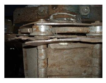
Picture shows damaged side wings on belt.
