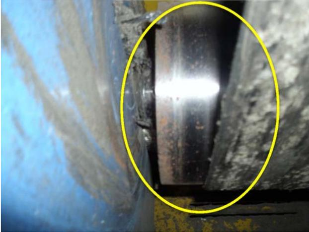
Head and tail pulley needs to be replaced. Belt tracking is pulling to the right.
