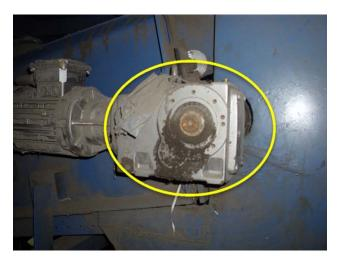
Gearmotor is leaking. It is held stable by zip ties. Replacement required.
