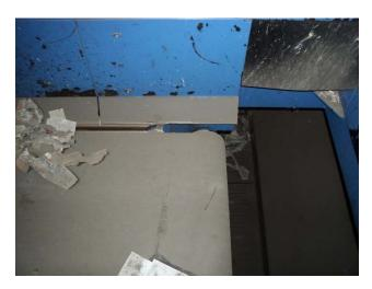
Belt is worn, tracking is off, replacement required.
