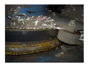
$Guards\ are\ omitted/missing,\ motor\ is\ leaking,\ replacement\ required.$
