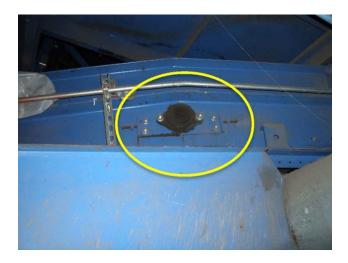
Bearings are worn/blown, replacement required.
