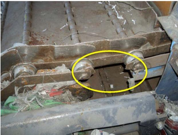
D hole bars are missing/broken.
