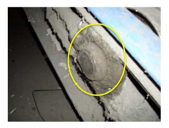
Bearings are worn/broken, replacement required.
