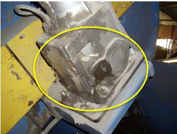
Gearmotors are leaking, replacement required.
