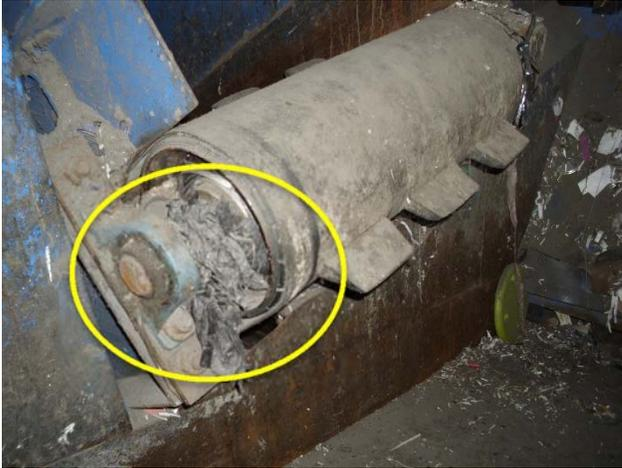
Condition of bearing is worn/blown. Replacement required.
