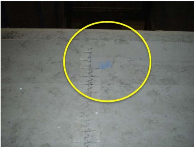
Belt is torn, lacing torn, replacement required.
