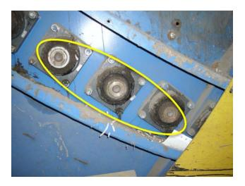
Bearings are worn and need to be replaced.
