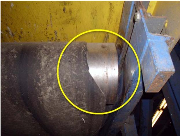
Belt is torn and tracking is veering to the left. Replacement required.
