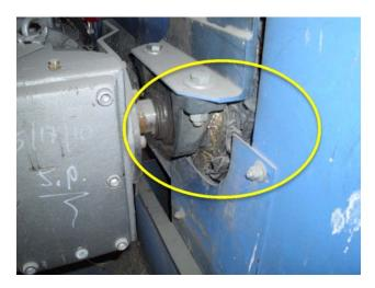
Picture above shows wrapped shaft, cleaning required. Material is building up under belt, causing more damage.
