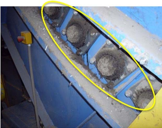
All bearings are worn and need to be replaced.
