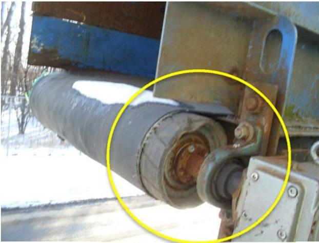
Pulley is damaged and needs to be replaced. Belt tracking is pulling to the left.
