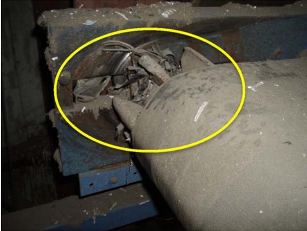
Conveyor pulley shaft is wrapped, bearing and pulley both need to be replaced. Belt is worn and replacement is required.
