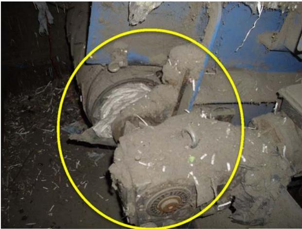
Severely wrapped head shaft, belt tracking is off, gearmotor is leaking. Replace all components.
