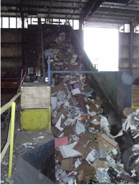
Amount of debris pile up has made it impossible for technician to properly inspect all aspects of the conveyor. It is said that the rails/tracks are worn, head shaft is bent and belt is in bad condition. Replacement of these components would optimize use of conveyor.
