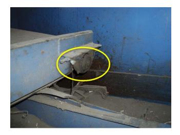
Bearing is worn, replacement required.
