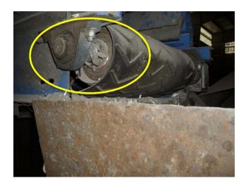
Pulleys and bearings are damaged, replacement required.
