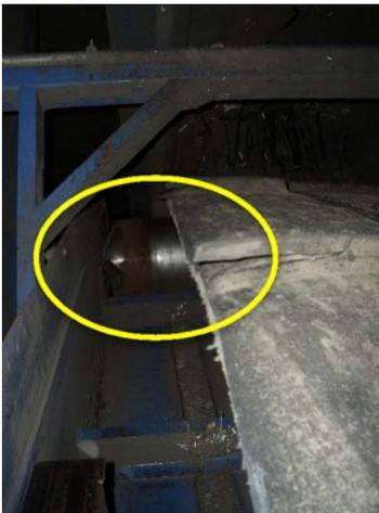
Belt tracking and tensioning completely off to the right.
