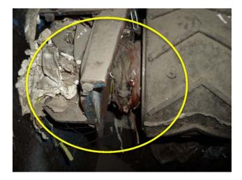
Pulleys are wrapped, replacement required.
