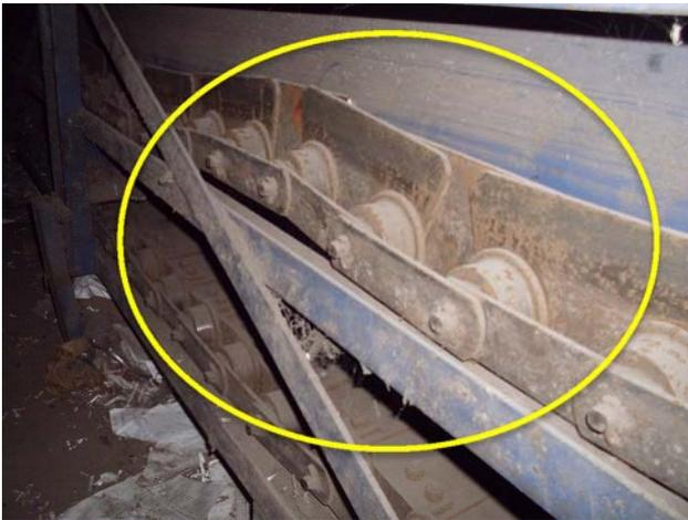
Belt needs to be replaced, tensioning is off as well.
