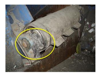
Condition of bearing is worn/blown. Replacement required.
