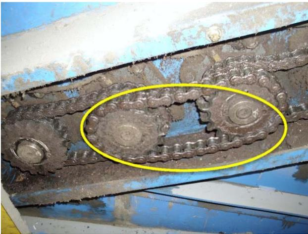
Chains are stretched/worn, full replacement needed. Sprockets are worn, replacement needed.
