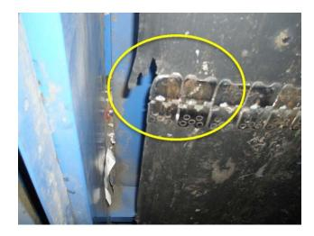
Belt is torn, laced improperly. Replacement recommended.
