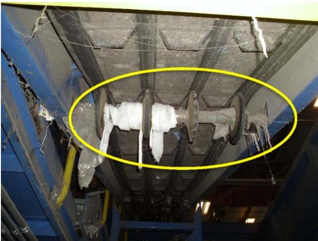
Return rollers are worn and wrapped. Replacement required.
