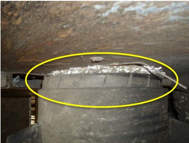
Picture shows belt tracking being off.
