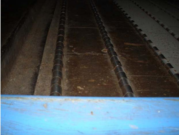
Conveyor is in good condition. Cleaning required for optimal use.
