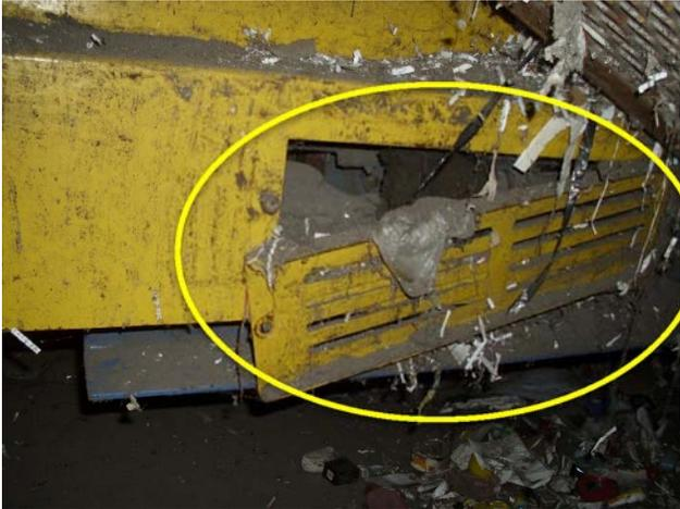
Guarding has been removed and left open. Pulleys are exposed, shows signs of severe wear, replacement required.
