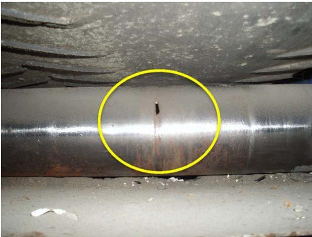
Return rollers are damaged. Replacement required.
