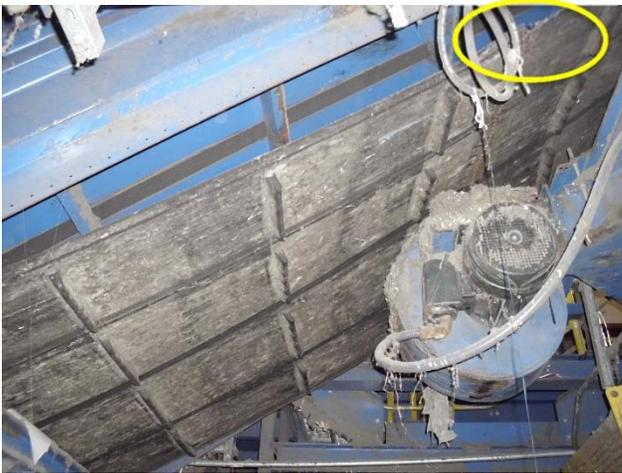
Belt is torn and needs to be replaced. Tensioning is lacking.
