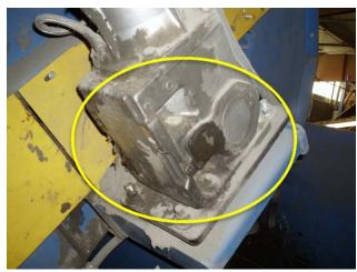
Gearmotors are leaking, replacement required.
