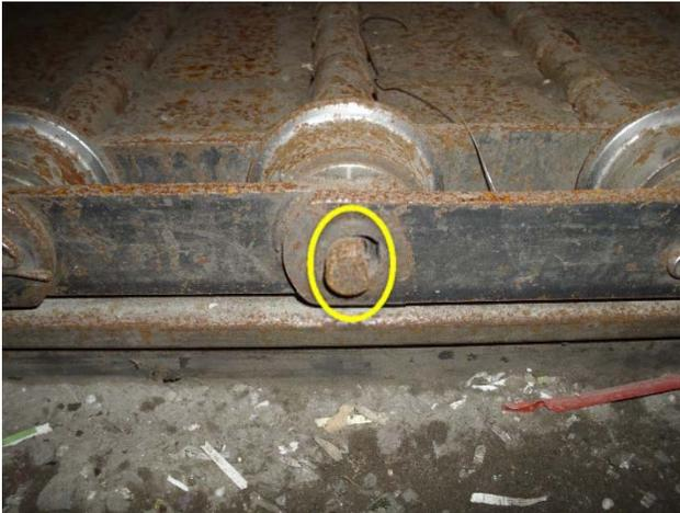
D hole bars are worn out, no cotter pin installed.
