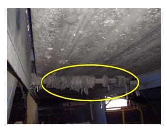
Return rollers are wrapped and worn, replacement required.
