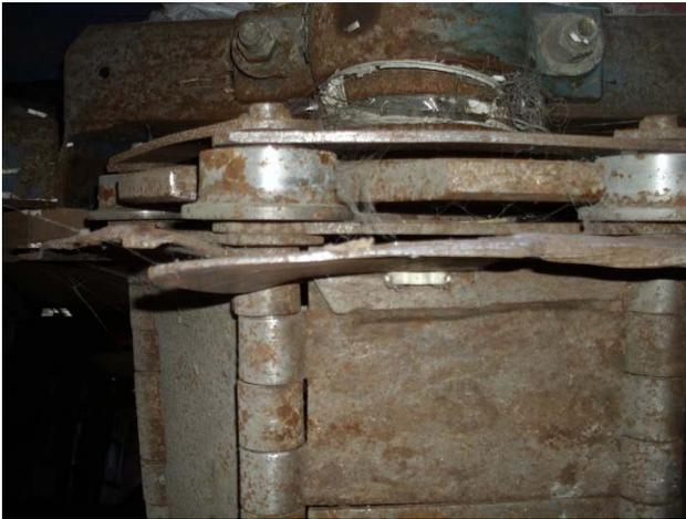
Picture shows damaged side wings on belt.
