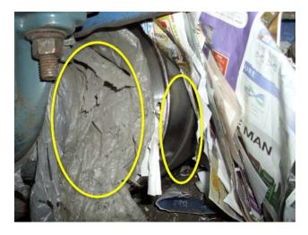
Shaft is wrapped, belt tracking needs to be corrected.
