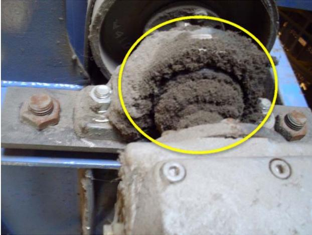
Bearings are worn and needs to be replaced.
