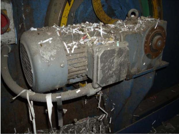
Equipment needs much work to be fully functional. Bearings needs to be replaced, proper cleaning required, guards are also omitted/missing.
