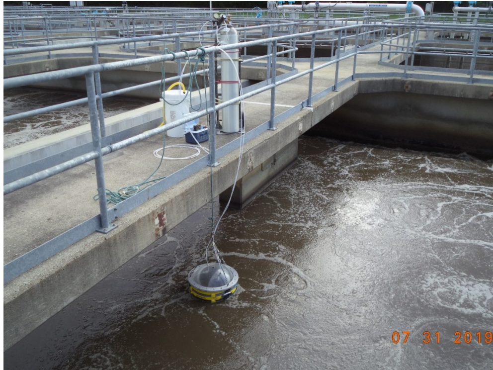
Figure 3-1. Summer Sampling Using EPA Flux Chamber
