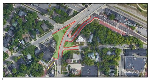
Figure 12: Option D: Variation on Option C. Maintains 2-way movements for Carey, eliminates Summit to Detroit and Division to Summit movements.
