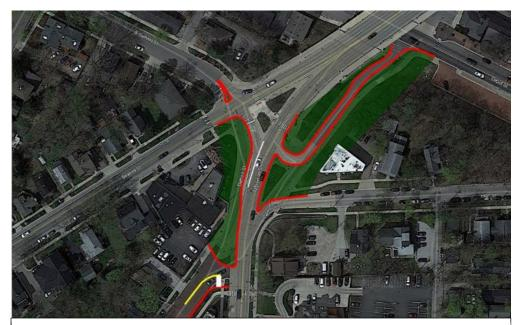
Figure 11: Option C – Close northbound entrance to Carey St from Division St and southbound access to Detroit St from Broadway St/Summit St. Maintains access from Division to Summit. Would maintain access to the Broadway Street bridge from Depot Street and to High Street from Division.
