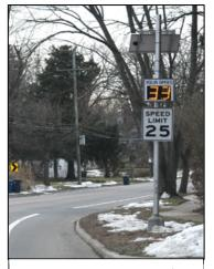
Figure 4: Example of radar-based speed warning system.
