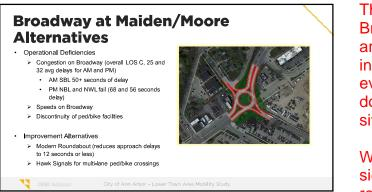
The last specific location we considered was Broadway at Maiden Ln and Moore St. There are significant delays at this signalized intersection, especially in the morning and evening commute times. Retiming the signal does not hold any promise of improving this situation.
