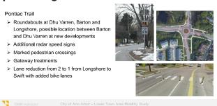
Here are the specific recommendations for speed management in the Pontiac Trail corridor. This slide notes the type of treatments being proposed and the following two show the locations where they should be provided.
