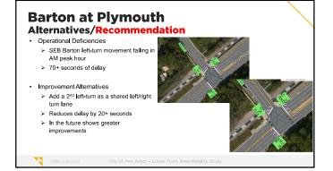
At Barton and Plymouth, the very high left turn demand from EB Barton to NE bound Plymouth is an issue. This causes very long delays, especially in the a.m. commuter peak.
