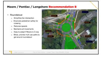
The longer term answer is to simplify the geometry by constructing a single lane roundabout. This may be desired especially if the City wishes to convert Moore St from one-way to two-way traffic movements. Depicted is a roundabout concept that works with Moore carrying two-way traffic.
