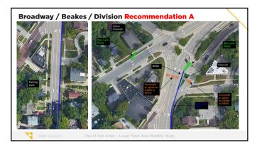
We recommend that the City initially focus on improving pedestrian and bicycle safety. The third travel lane for NB Division (west curb lane) should be relegated to a narrow parking lane and the surplus space used to carry the on-street bike lane further to the north to just short of the Broadway bridge.
