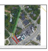
Finally, we looked at the remaining portion of Pontiac Trail and its connection with Swift St. Pontiac Trail pavement can be narrowed to provide the space to add sidewalk and a on-street bike lane.
