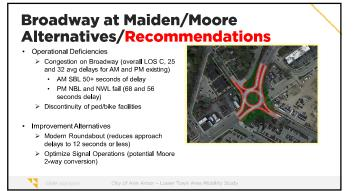
We then considered the appropriate treatment for Broadway at Maiden Ln and Moore St. There are significant delays at this signalized intersection, especially in the morning and evening commute times. Retiming the signal does not hold any promise of improving this situation.
