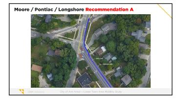
We recommend as an initial improvement that lane widths on Moore be reduced. The extra space would be to provide a on-street bike lane, which could wrap around the corner and link up with the existing one on Pontiac Trail. Rather than the current free flow movement of Moore turning right onto Pontiac Trail, this would be put under the control of a Yield sign. The overhead flashing beacons would be removed.
