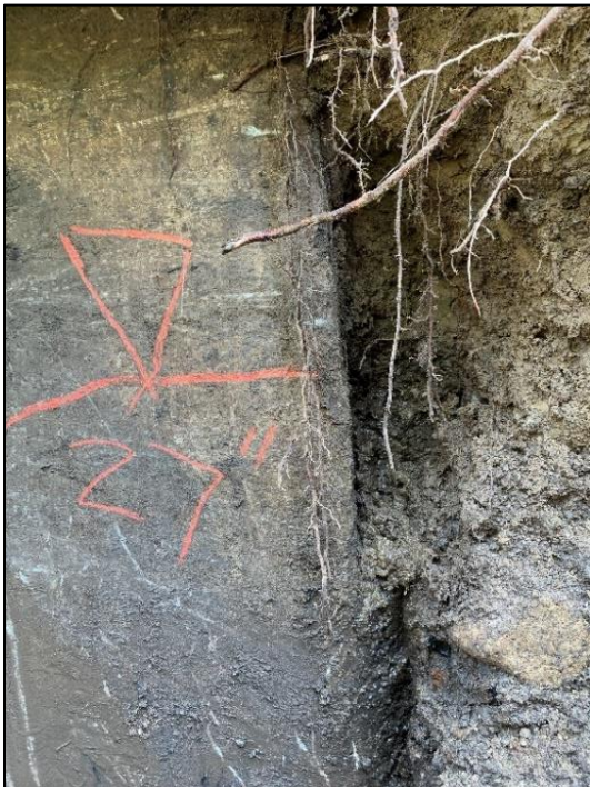
Photo 2: High Ground Water Table at 27" Below Grade
