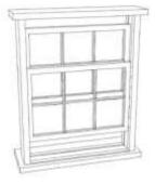
Double-Hung: Α window with two sashes, each movable vertically by means a sash cord and weights, or some other mechanism. Double-hung windows are the most common.
