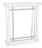
**Fixed**: A fixed frame window (or part thereof) that does not open. Fixed windows have sash that are permanently fixed to the frame. They are often flanked by double-hungs or
