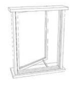
Casement: A single window sash that opens on hinges fixed to its vertical edge. The casement window's full-height opening provides excellent ventilation. Casements, especially wooden ones, can
