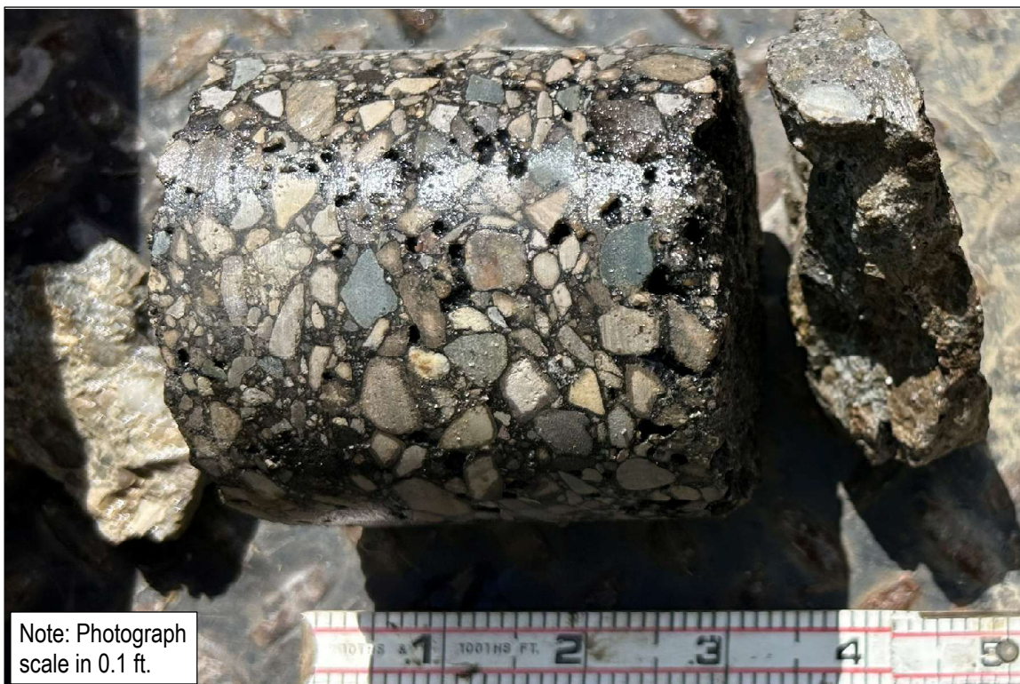
Photo 32: SB-2026-146 (Kingsley St.): 3.5-inch Asphalt, 2-inch Concrete
