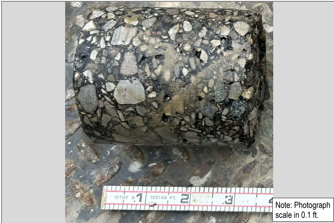
Photo 37: SB-2026-151 (Ingalls St.): 4-inch Asphalt, 3-inch Concrete (non-recoverable)
