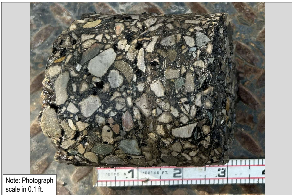
Photo 28: SB-2026-142 (Kingsley St.): 3.5-inch Asphalt, 5-inch Concrete (non-recoverable)
