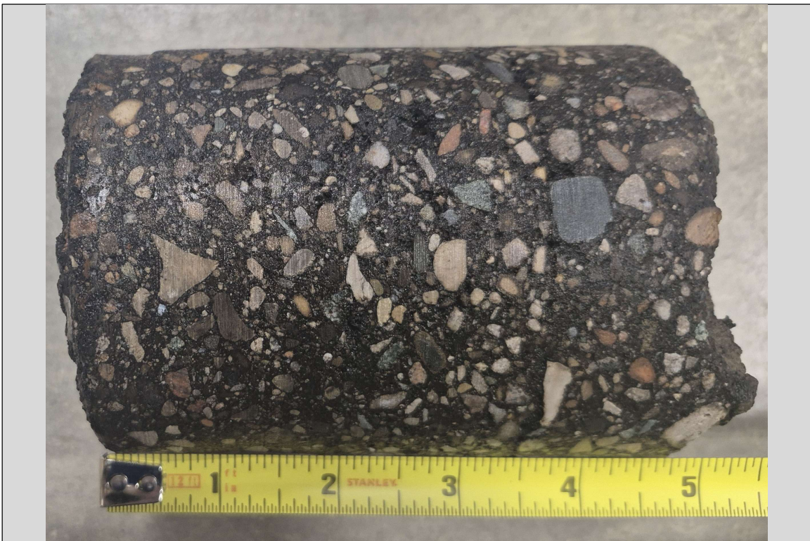
Photo 20: SB-2026-127 (S. Huron Pkwy., Arlington Square): 5-inch Asphalt
