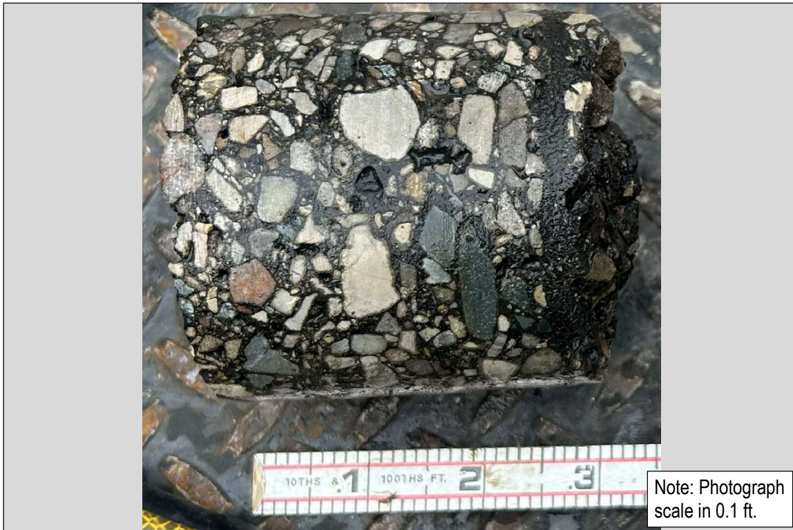
Photo 39: SB-2026-153 (Ingalls St.): 3.5-inch Asphalt, 3-inch Concrete (non-recoverable)
