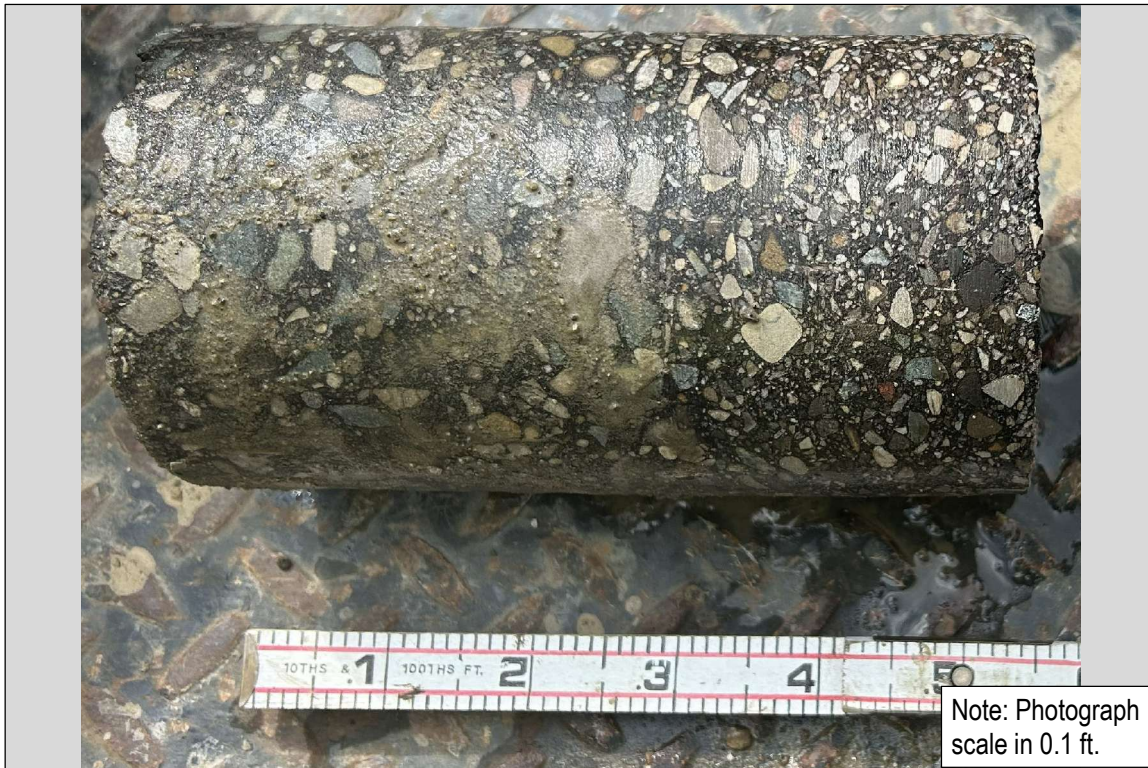
Photo 12: SB-2026-119 (Packard St.): 6.5-inch Asphalt
