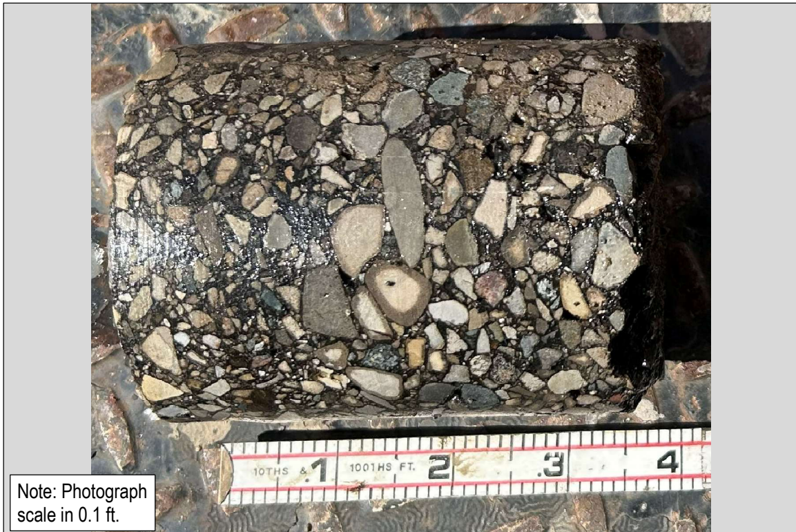
Photo 33: SB-2026-147 (Kingsley St.): 4-inch Asphalt
