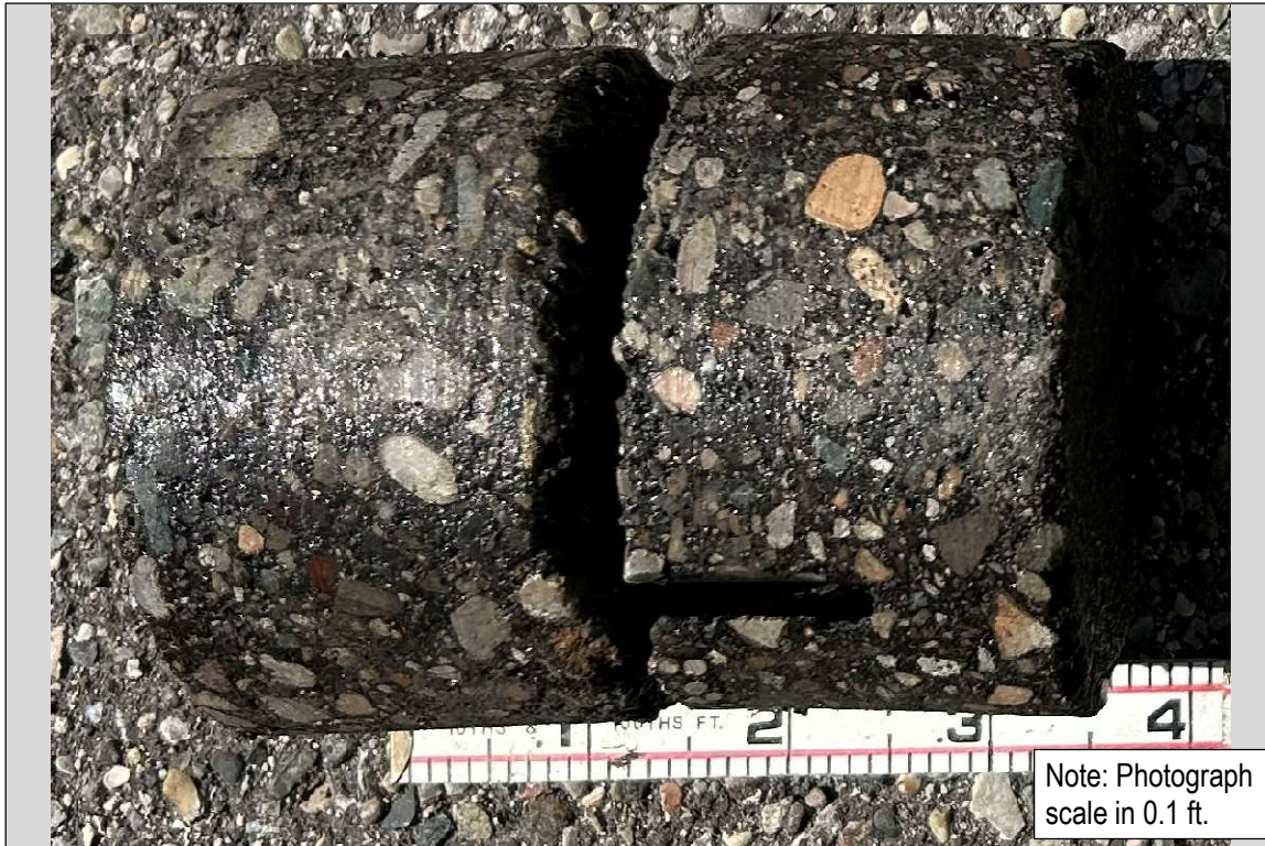
Photo 21: SB-2026-128 (S. Huron Pkwy., Arlington Place): 5-inch Asphalt
