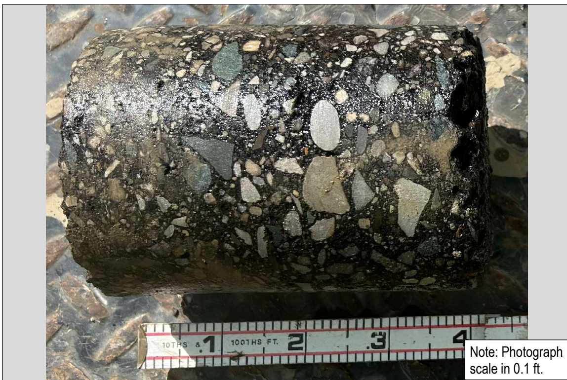
Photo 13: SB-2026-120 (Packard St.): 5-inch Asphalt
