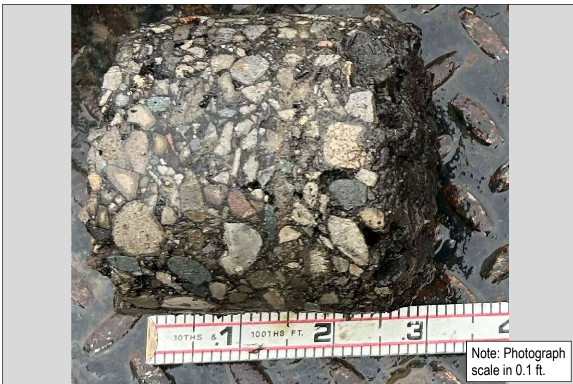
Photo 36: SB-2026-150 (Ingalls St.): 3.5-inch Asphalt
