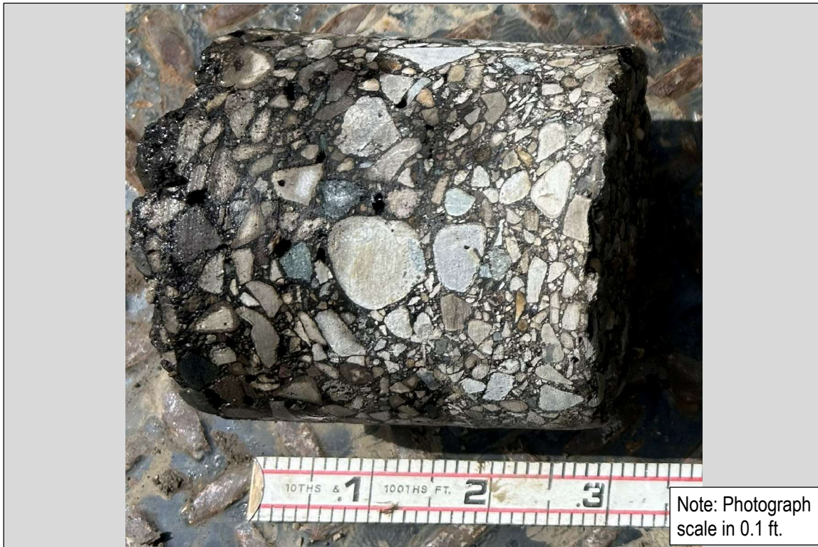
Photo 31: SB-2026-145 (Kingsley St.): 3.5-inch Asphalt
