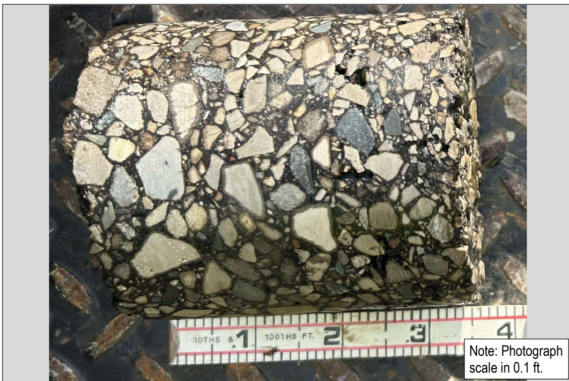
Photo 40: SB-2026-154 (Ingalls St.): 4-inch Asphalt, 3-inch Concrete (non-recoverable)
