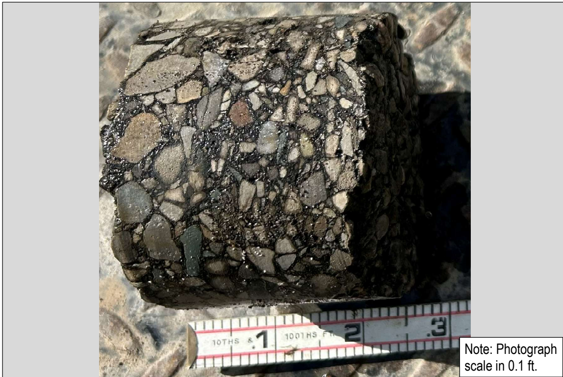
Photo 29: SB-2026-143 (Kingsley St.): 3-inch Asphalt, 5-inch Concrete (non-recoverable)
