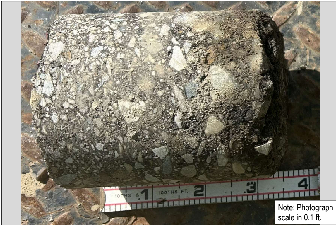
Photo 14: SB-2026-121 (Packard St.): 4-inch Asphalt
