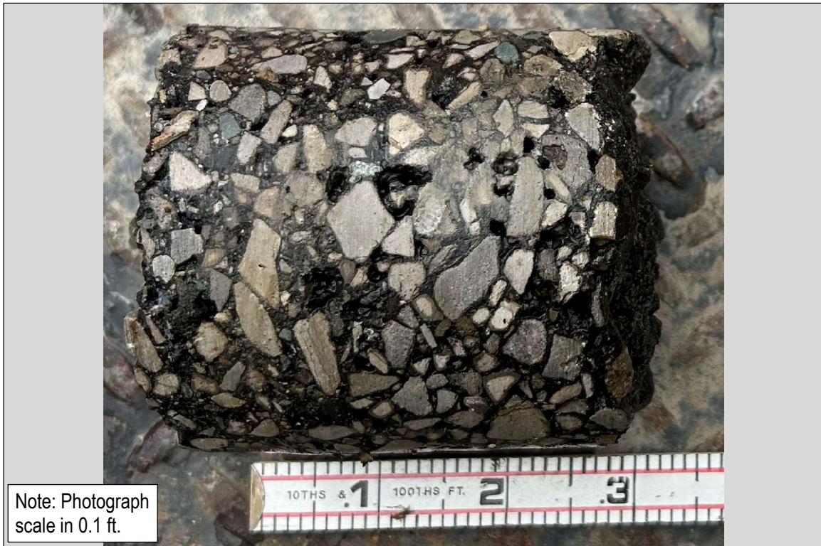
Photo 27: SB-2026-141 (Kingsley St.): 3.5-inch Asphalt
