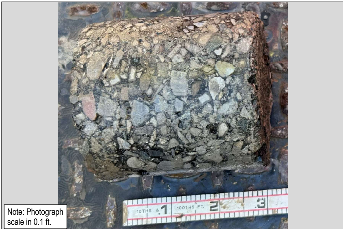
Photo 34: SB-2026-148 (Ingalls St.): 3.5-inch Asphalt
