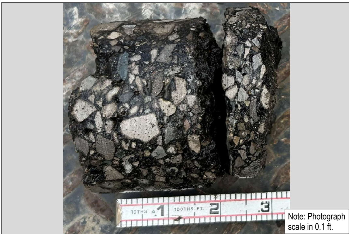
Photo 26: SB-2026-140 (Kingsley St.): 3.5-inch Asphalt
