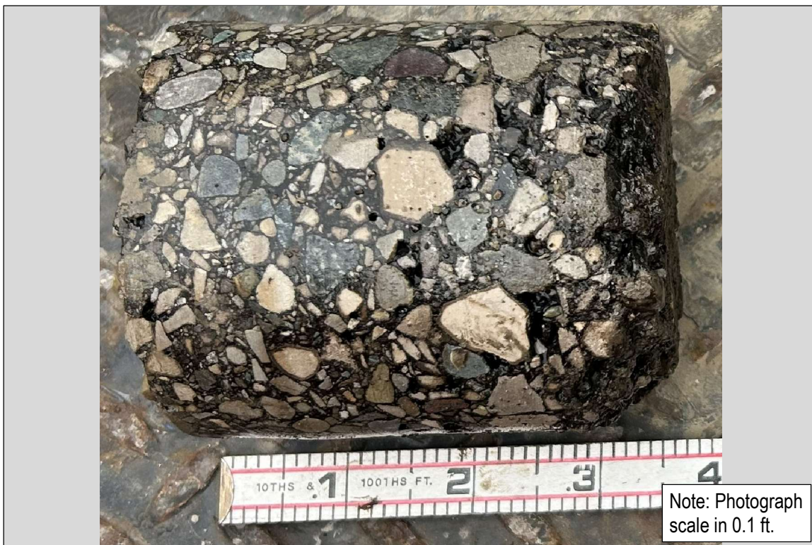
Photo 38: SB-2026-152 (Ingalls St.): 4-inch Asphalt, 3-inch Concrete (non-recoverable)
