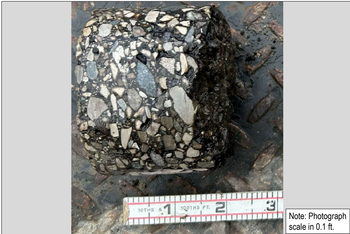
Photo 25: SB-2026-139 (Kingsley St.): 3-inch Asphalt
