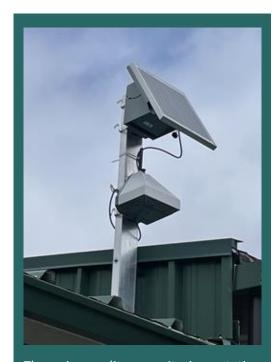
The air quality monitoring station located at the Ann Arbor Farmers Market in Kerrytown. Each of our monitoring systems is 100% solar powered and transmits data via cellular networks. Pollutants measured include carbon monoxide, carbon dioxide, ozone, particulate matter, nitric oxide, nitrogen dioxide, and sulfur dioxide. Temperature, humidity, and pressure data are also collected.
