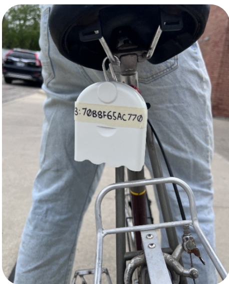
A small, portable air quality monitor attached to a bike seat.
