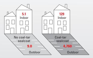
PAH-contaminated dust on coal-tar-sealcoated pavement (right) is tracked indoors.<sup>10</sup> Concentrations shown are median values for the sum of the 16 Priority Pollutant PAHs, in units of milligrams per kilogram, in house dust and parking lot dust.
