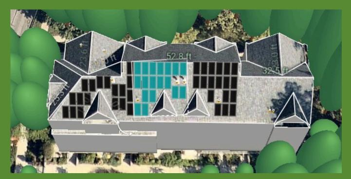
Above is the solar plan as drafted by the solar installation company.
