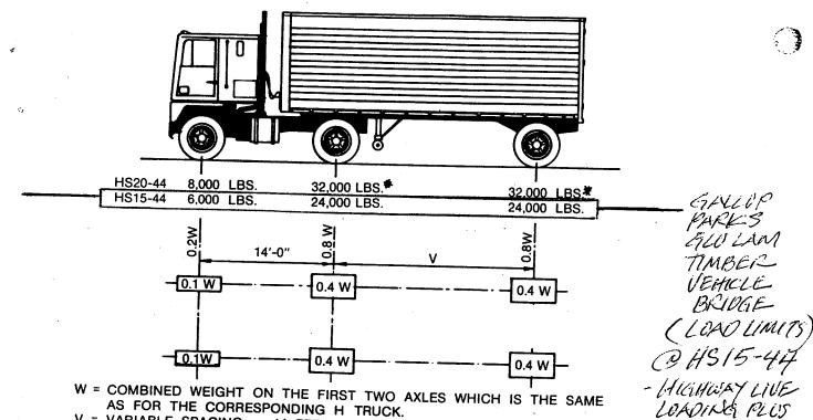
V = VARIABLE SPACING - 14 FEET TO 30 FEET INCLUSIVE. SPACING TO BE USED IS THAT WHICH PRODUCES MAXIMUM STRESSES.
