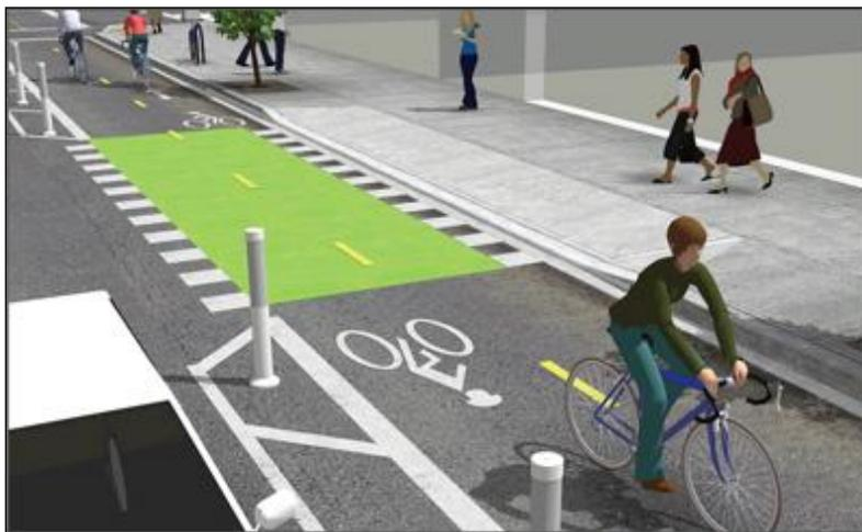
*Figure 8 – NACTO Urban Bikeway Design Guide Two-Way Cycle Track Illustration*
