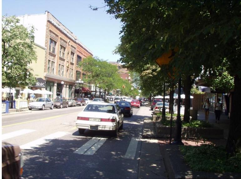
Curbs prevent water in the street gutters from entering the pedestrian space, discourage vehicles from driving over the pedestrian area, and make it easy to sweep the streets. In addition, the curb helps to define the pedestrian environment within the streetscape, although other designs can be effective for this purpose. At the corner, the curb is an important tactile element for pedestrians who are finding their way with the use of a cane.
