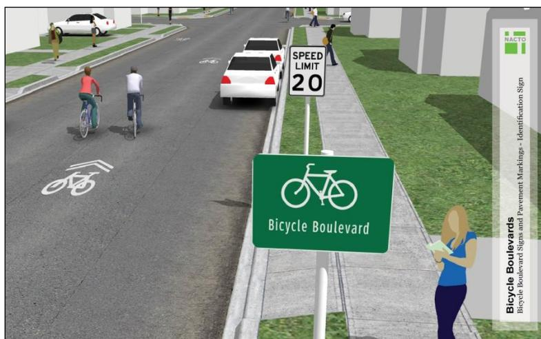
Figure 7 – NACTO Urban Bikeway Design Guide Bicycle Boulevard: Signs and Pavement Markings
