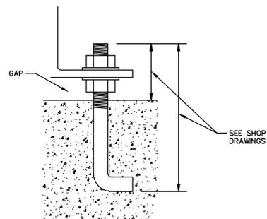
ANCHOR BOLT PROJECTION DETAIL
