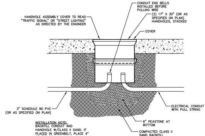
DOUBLE STACK HANDHOLE DETAIL
