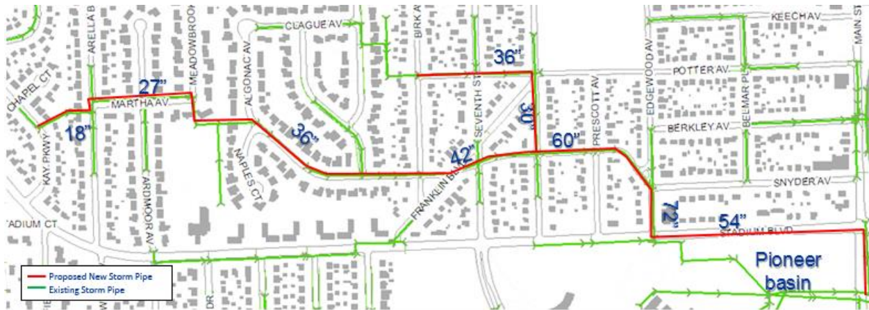
Figure 4-7 – Conceptual Layout of Conveyance Alternative for Edgewood/Snyder
