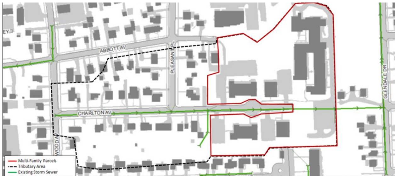
Figure 4-36 – Conceptual Layout for Upstream Detention Alternative for Glendale/Charlton
