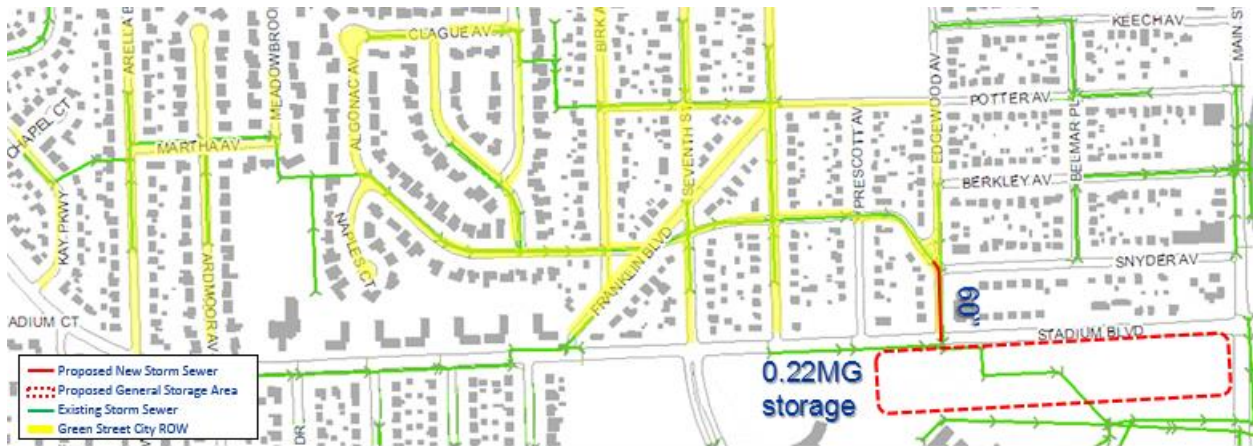
Figure 4-5 – Conceptual Layout of Green Streets Alternative for Edgewood/Snyder
