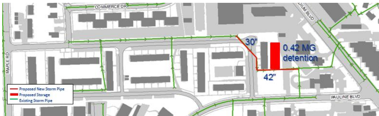
Figure 4-10 – Conceptual Layout for Storage Alternative at Park Place Apartments
