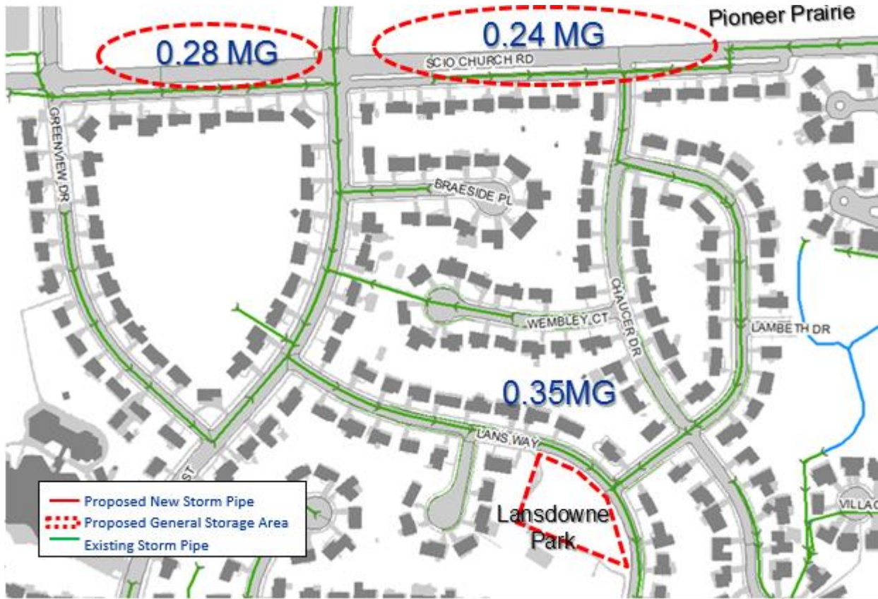
Figure 4-31 – Conceptual Layout for Storage Alternative for Scio Church / S. Seventh Street
