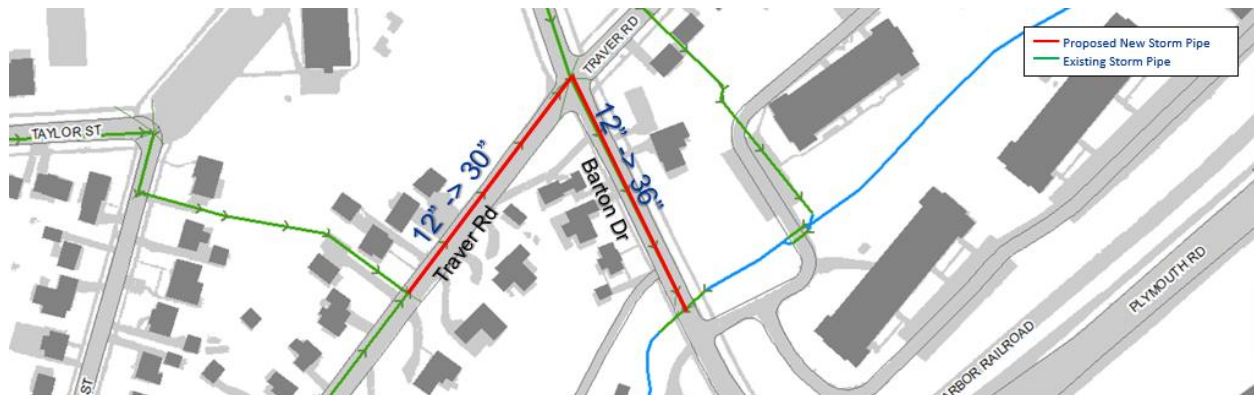
Figure 4-54 – Conceptual Layout for Conveyance Improvement Alternative for Traver/Barton
