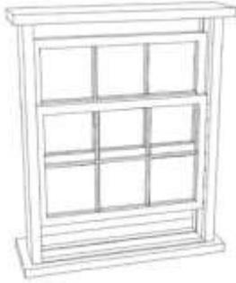
**Double-Hung:** A window with two sashes, each movable vertically by means a sash cord and weights, or some other mechanism. Double-hung windows are the most common.
