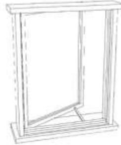
**Casement:** A single window sash that opens on hinges fixed to its vertical edge. The casement window's full-height opening provides excellent ventilation. Casements, especially wooden ones, can suffer damage if left open to the elements.
