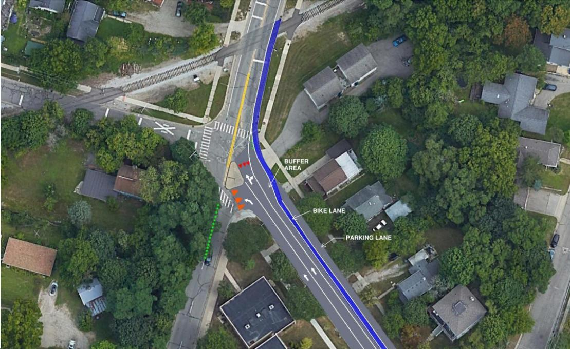
**Figure 16: Short Term Option 2: Restripe Moore St to narrow travel lanes to +11' to add a bicycle lane adjacent to the parking lane (northeast curb). Carry the new bike lane onto NB Pontiac Trail, joining existing north of RR tracks. Change intersection control for Moore at Pontiac to YIELD.**
