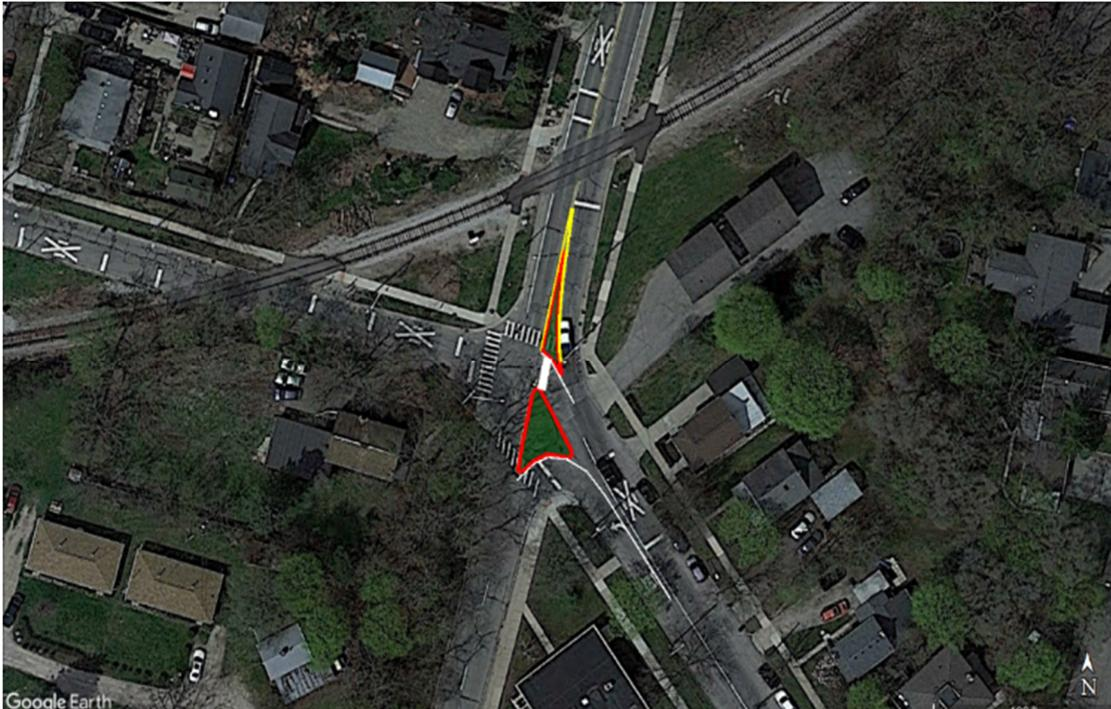
**Figure 17: Option A – Add new islands to intersection. An added stop sign would be provided for the Moore Street to Longshore Drive movement. The overhead beacons would be removed in favor of adding RRFB’s for the Pontiac Trail pedestrian crossing.**
