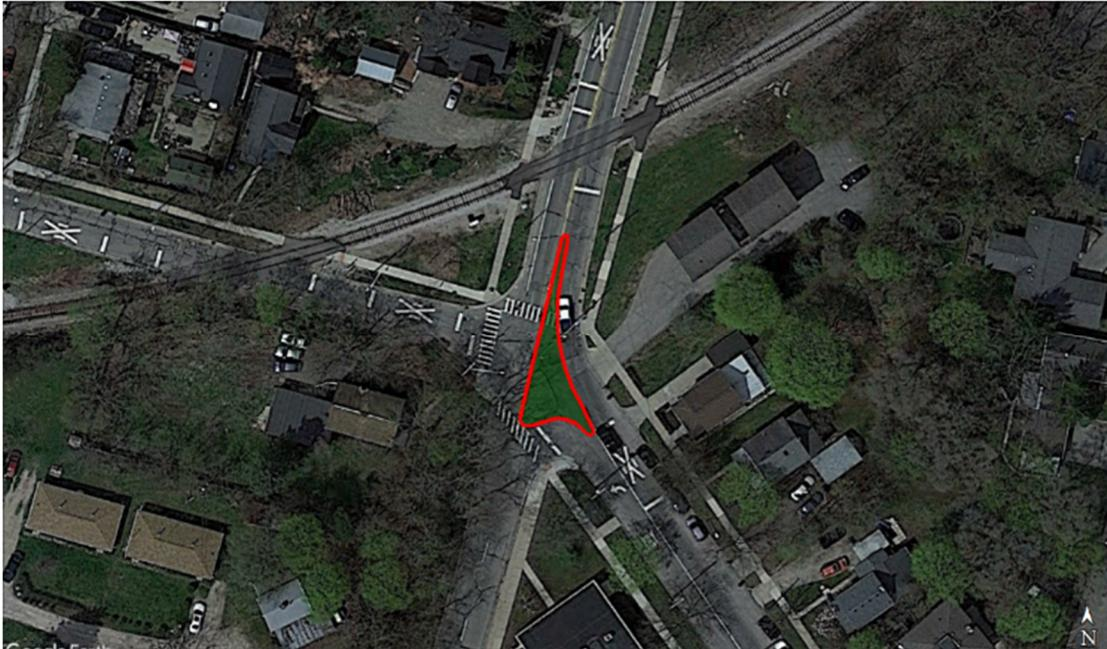
**Figure 18: Option B – Add new island to intersection. Treatment would simplify the intersection by allowing only two movements from Moore Street and require Longshore to be right in/out only. Would remove intersection beacons.**
