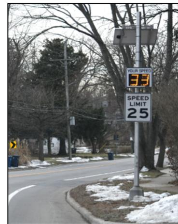
**Figure 4: Example of radar-based speed warning system.**
