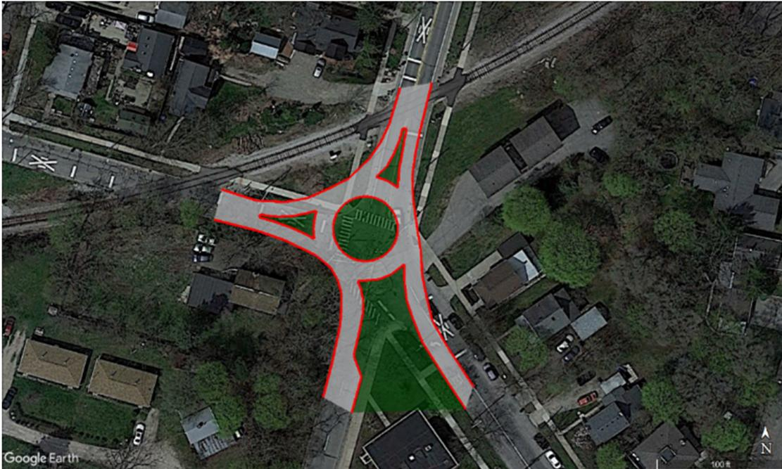
**Figure 19: Option C – Reconfigure intersection as one-lane roundabout. Maintains access for all existing movements. Would eliminate the intersection beacons. Depicted is a roundabout with about 90' outside diameter.**
