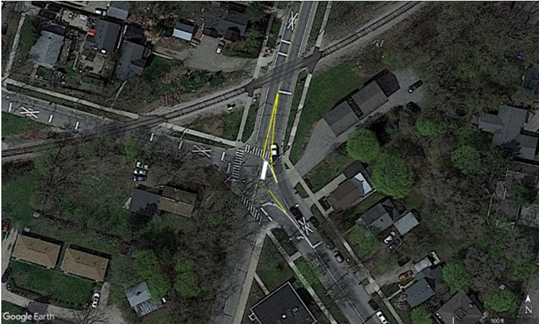
**Figure 15: Short Term Option 1: Add pavement markings to better delineate vehicle paths through intersection. Maintain existing signals, but swap flashing yellow circular light for flashing yellow right arrow.**
