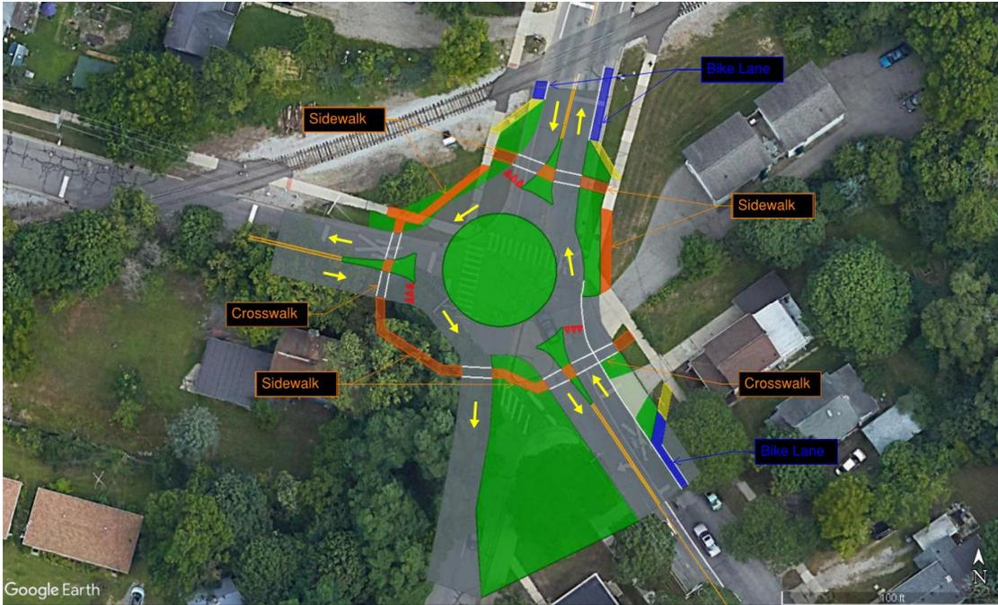
**Figure 20: Option D – Same as Option C but facilitating two-way movements on Moore St. Reconfigure intersection as one-lane roundabout. Maintains access for all existing movements. Would eliminate the intersection beacons. Depicted is a roundabout with about 90’ outside diameter.**
