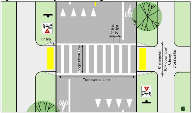
Fig. 2.4AB. Ladder Style Crosswalk Design Guidelines
