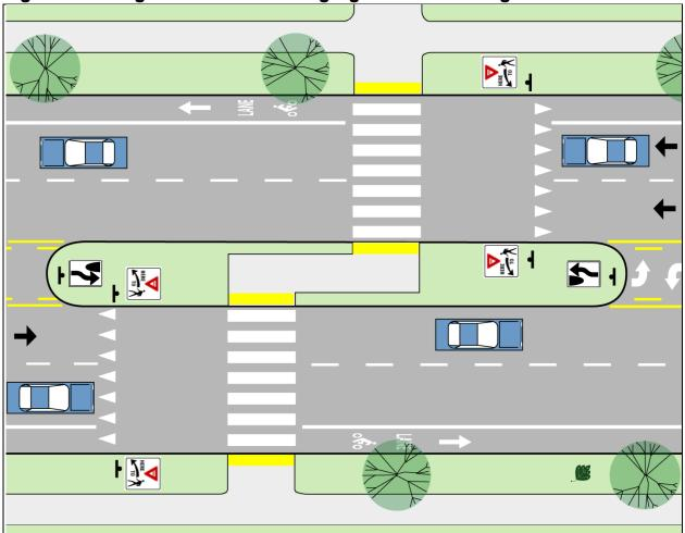
Fig. 2.4Z. Unsignalized Mid-block Zigzag Crosswalk Design Guidelines
