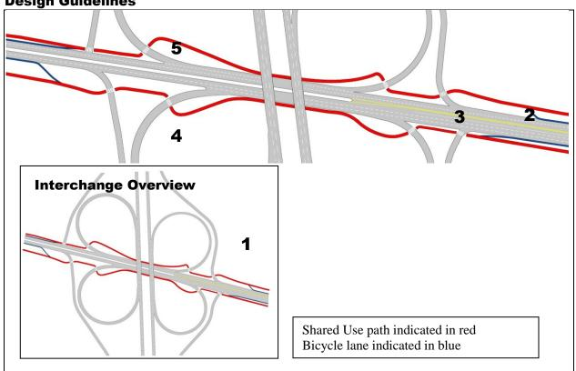
Fig. 2.4L. Urban Free-flow Underpass Interchange Retro-fit Design Guidelines
