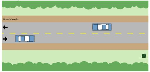
A rural cross-section (no curbs) with gravel or grass shoulder. The existing roadway travel lanes are not of a sufficient width to accommodate bicycle lanes by lane narrowing.
