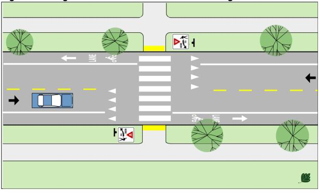
Fig. 2.4V. Unsignalized Basic Mid-block Crosswalk Design Guidelines
