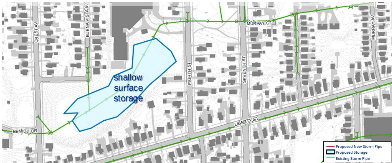
Figure 4-27 – Conceptual Layout for Surface Storage Alternative for Mulholland Ave
