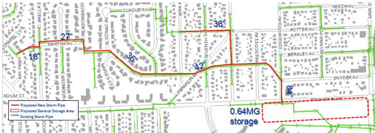
Figure 4-6 – Conceptual Layout of Storage Alternative for Edgewood/Snyder
