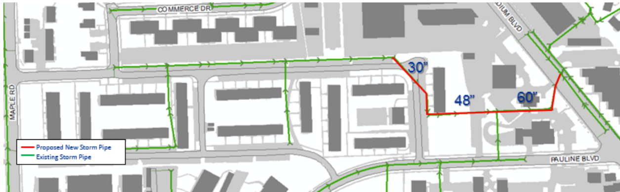
Figure 4-11 - Conceptual Layout for Conveyance Alternative at Park Place Apartments
