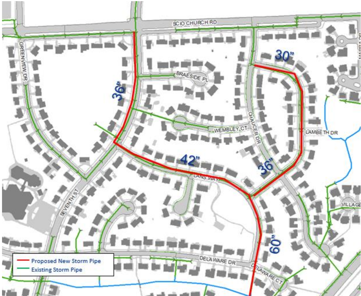
Figure 4-33 – Conceptual Layout for Conveyance Alternative for Scio Church / S. Seventh Street
