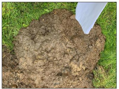
Photo 8: Saturated Excavated Spoil
