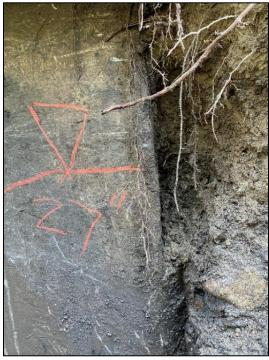
Photo 2: High Ground Water Table at 27" Below Grade
