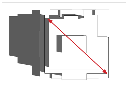
The maximum diagonal is the longest diagonal dimension of a building or tower.
