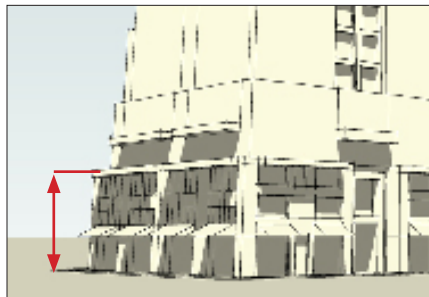
The streetwall is the wall formed by buildings along the setback line or the base portion of a taller building or tower. Streetwall height is the height of the streetwall portion of a building.
